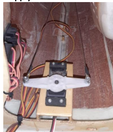
Above: the rudder servo can be installed on a plywood table glued with 30 to 40 minutes epoxy glue at the bottom of the fuselage in the case of using the pull-pull system.
