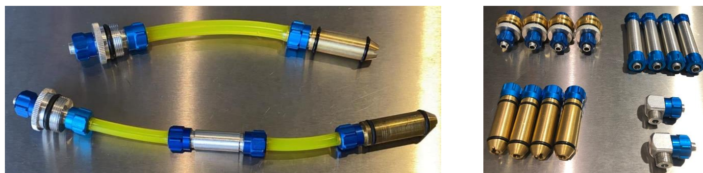
Above: clunk mounted without extender (above) and with clunk extender (below) to prevent hose bending (left) and complete connections including air vent manufactured by Rio Jets – sold separately (right).
