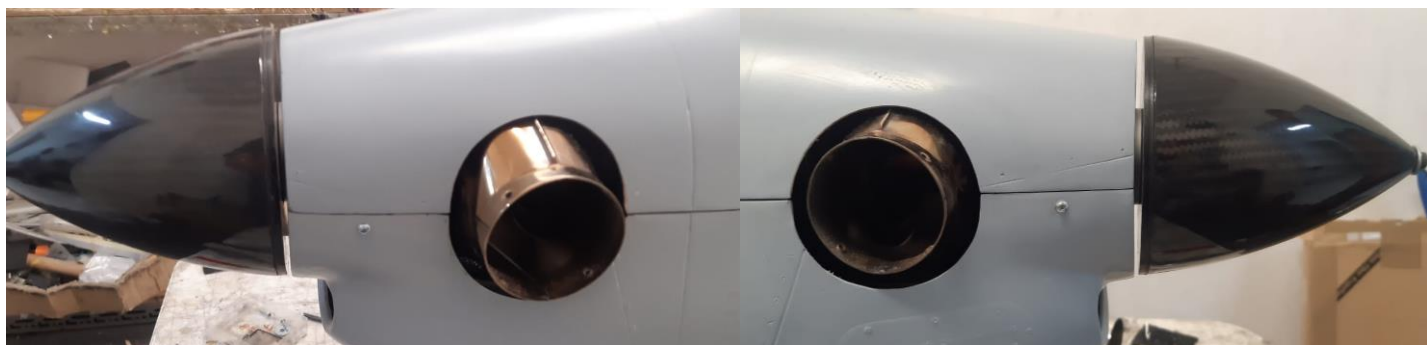
Above: correct alignment of the nose cowling with the spinner assembly and turbine exhausts holes.
