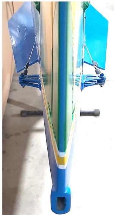
Above: pull-pull steel cables exits with Dubro heavy duty 4-40 ball links fixed on control horns with 4-40 screws and parlock nuts on both sides of the fuselage and rear view.
