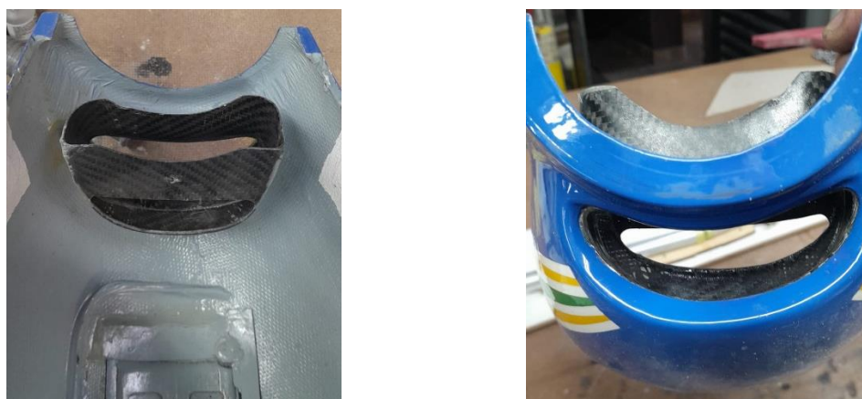
Above: : position of gluing the ventilation nozzle to the lower cowling.
