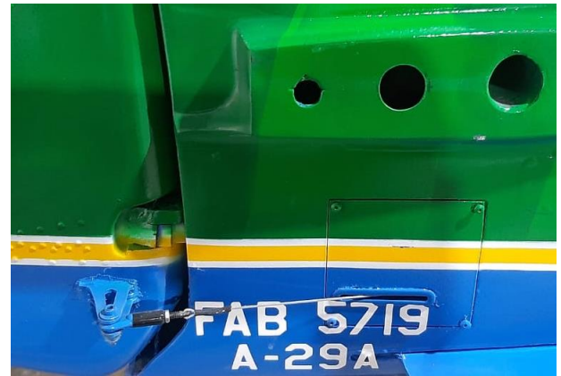
Above: pull-pull steel cables exits, with Dubro heavy duty 4-40 ball links fixed on control horns with 4-40 screws and parlock nuts on both sides of the fuselage.
