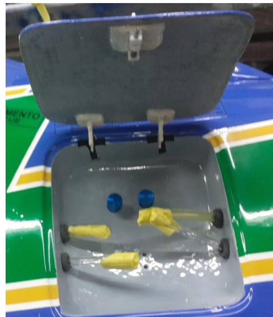
Above: door with installed hinges and latch in closed position (left) and open (right).
