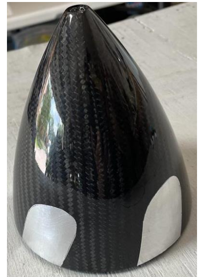
Above: spinner cut sequence to install the 5-blade propeller using equal shape adhesives.
