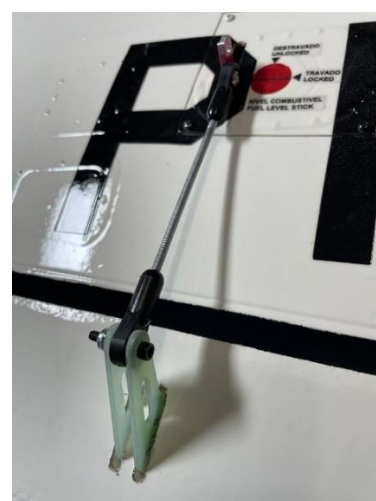
Above: aileron and flaps horns gluing process. Open slots (left), horns position with installed linkage (center) and glued horns on aileron command surface (right).
