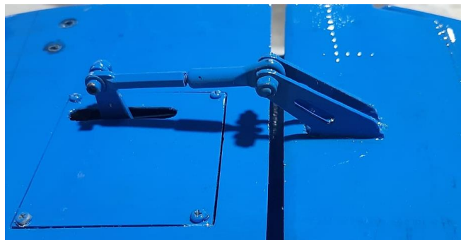
Above: elevators servos, servo arms and horns position with linkage.
