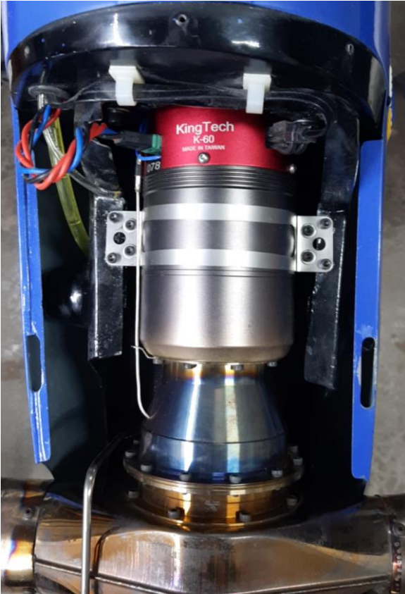
Above: turbine position on the carbon fiber turbine mount and lubrication tube position.
