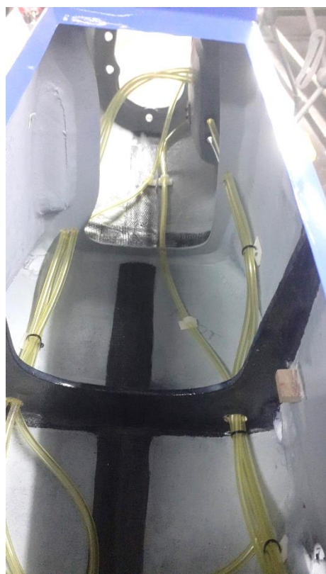
Above: installation of the fuel hoses in the fuselage with connections in the side door of the fuselage seen from the front of the fuselage (left and center) and from the rear of the fuselage (right).
