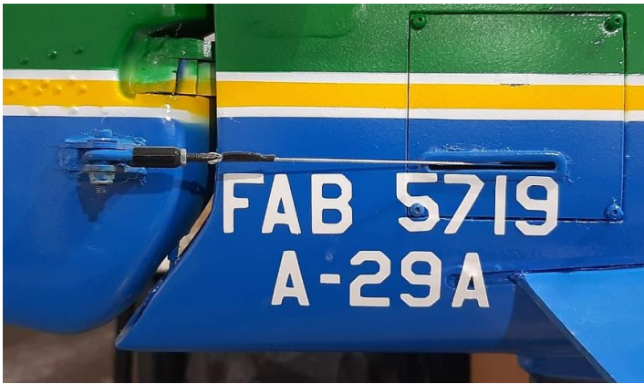
Above: pull-pull steel cables exits, with Dubro heavy duty 4-40 ball links fixed on control horns with 4-40 screws and parlock nuts on both sides of the fuselage.
