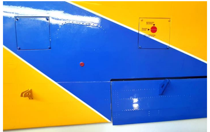
Above: location of the 40mm x 40mm reinforcements for fixing the horns on the right wing (left photo) and positioned and glued horns on the left wing (right photo).
