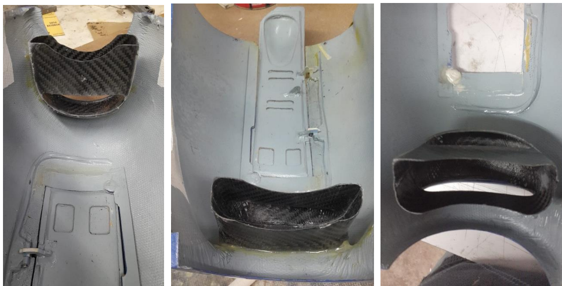
Above: position of gluing the ventilation nozzle to the lower cowling and the cutout at the rear of the nozzle to allow the passage of part of the air flow directly to the rear.
