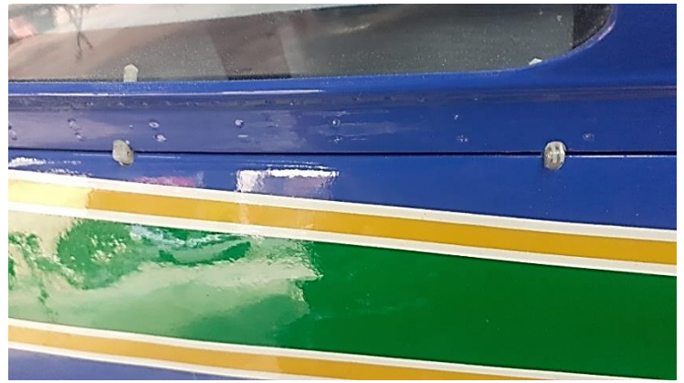
Above: canopy assembly hinges on fuselage (left) and in position for gluing to fuselage and canopy frame (right).
