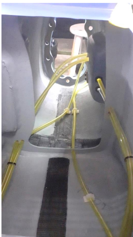
Above: installation of the fuel hoses in the fuselage with connections in the side door of the fuselage seen from the front of the fuselage (left and center) and from the rear of the fuselage (right).
