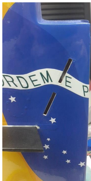
Above: right side of the original vertical stabilizer without cuts (left), cuts on the left side of the vertical stabilizer to allow the installation of formation lights (center) and LEDs properly installed (right).
