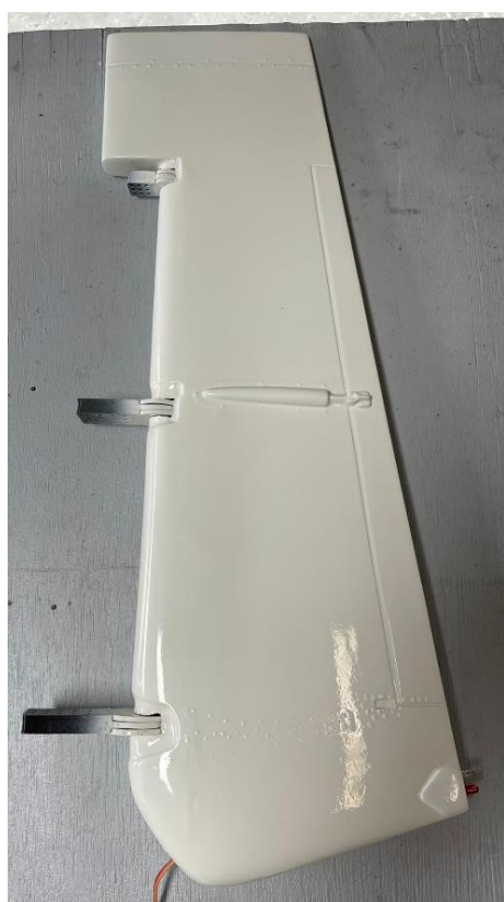
Above: rudder with glued hinges (left), housing for hinges on the vertical stabilizer (center) and rudder glued and installed (right).
