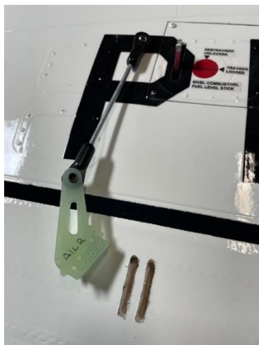
Above: aileron and flaps horns gluing process. Open slots (left), horns position with installed linkage (center) and glued horns on aileron command surface (right).
