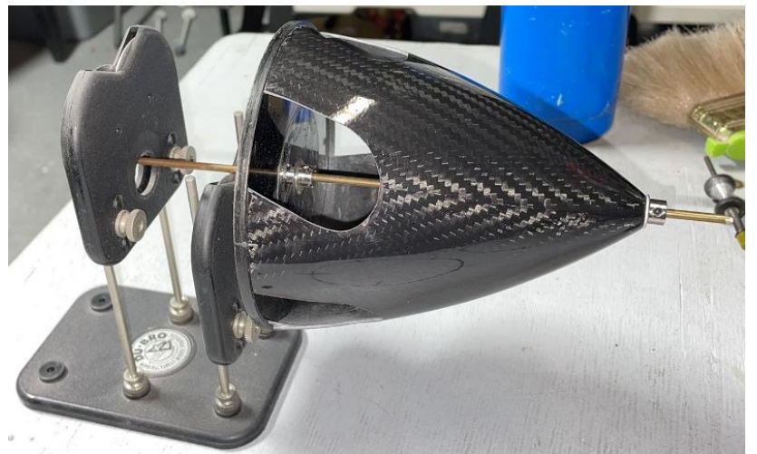
Above: spinner cut sequence to install the 5-blade propeller using equal shape adhesives (left) and spinner balancing to guarantee minimum vibration level to the spinner/propeller set (right).
