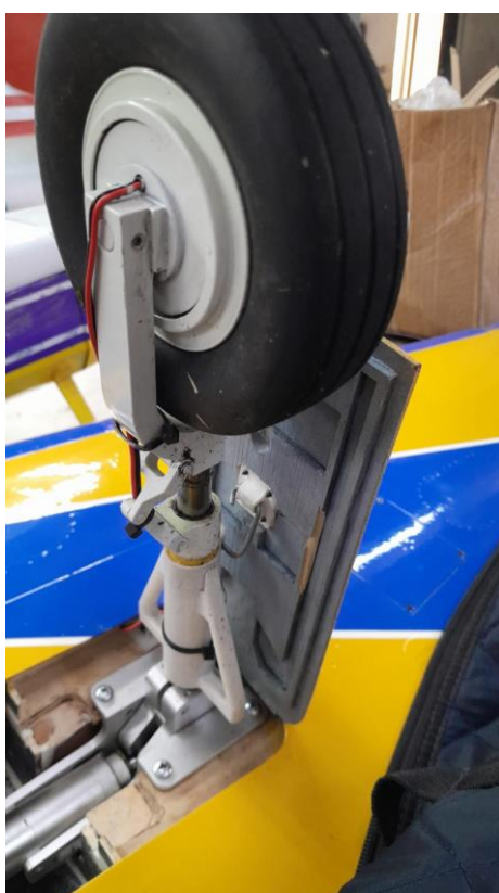
Above: external main landing gear door and hinges position on wing with landing gear door linkage.
