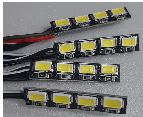
Above: fuselage dorsal beacon (left), fuselage intercept headlight (center) and vertical stabilizer formation lights (right)
