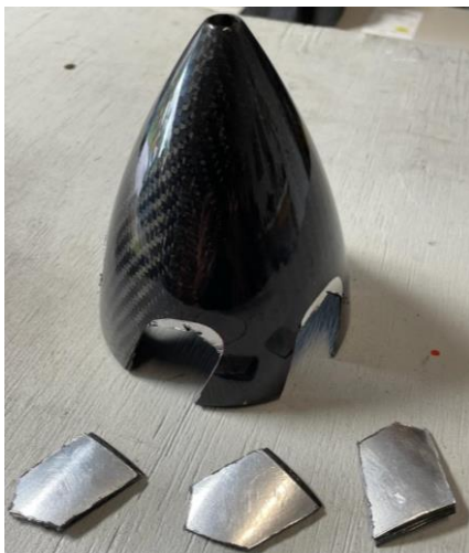
Above: spinner cut sequence to install the 5-blade propeller using equal shape adhesives (left) and spinner balancing to guarantee minimum vibration level to the spinner/propeller set (right).
