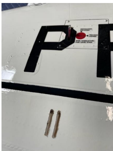
Above: aileron and flaps horns gluing process. Open slots (left), horns position with installed linkage (center) and glued horns on aileron command surface (right).
