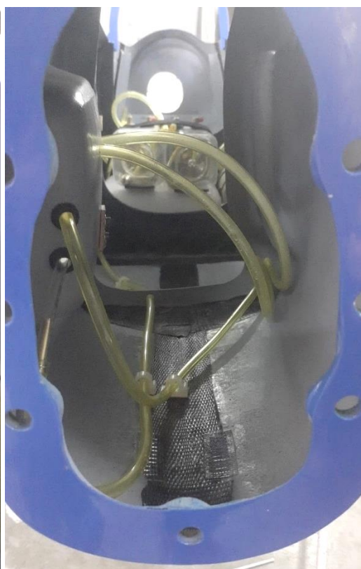
Above: installation of the fuel hoses in the fuselage with connections in the side door of the fuselage seen from the front of the fuselage (left and center) and from the rear of the fuselage (right).
