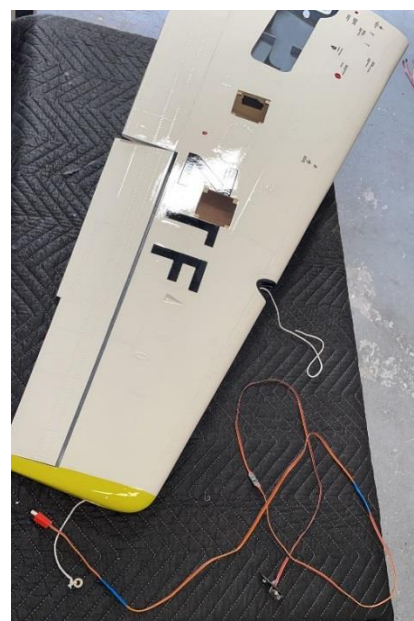
Above: weight on thread tip to pass the wires and wire to pull the wing landing light boards.
