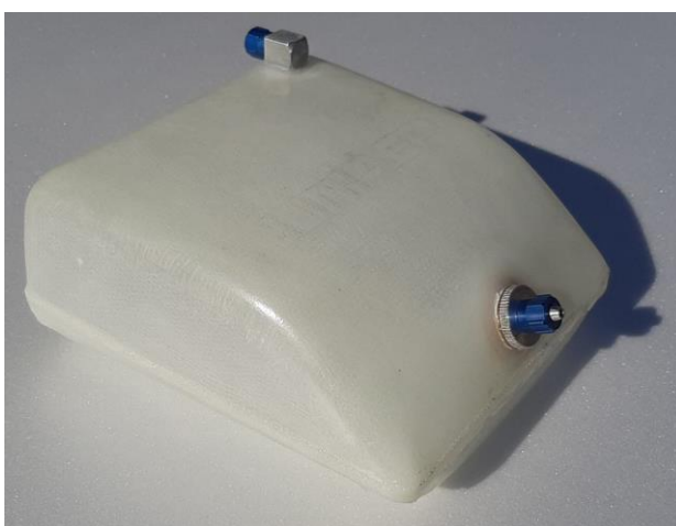
Above: fuel tank with Rio Jets nozzle and air vent installed and clunk assembly with extender and cover (left) and fully assembled fuel tank ready for installation on model airplane (right).
