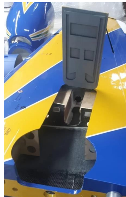
Above: external main landing gear door and hinges position on wing.
