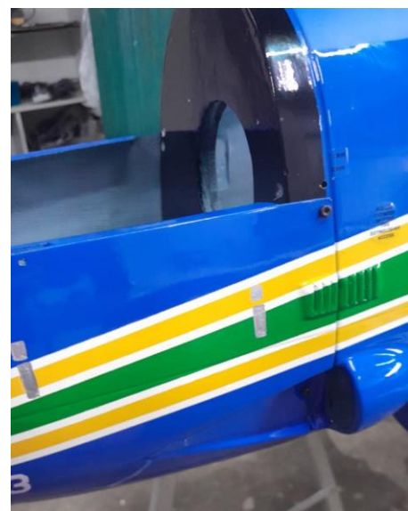
Above: markings of the 4 holes for fixing the turbine mount in the central part of the firewall and 9 holes for fixing the cowling with stud bolts at the ends of the firewall (left and center) and lower fairing attached to the fuselage (right).
