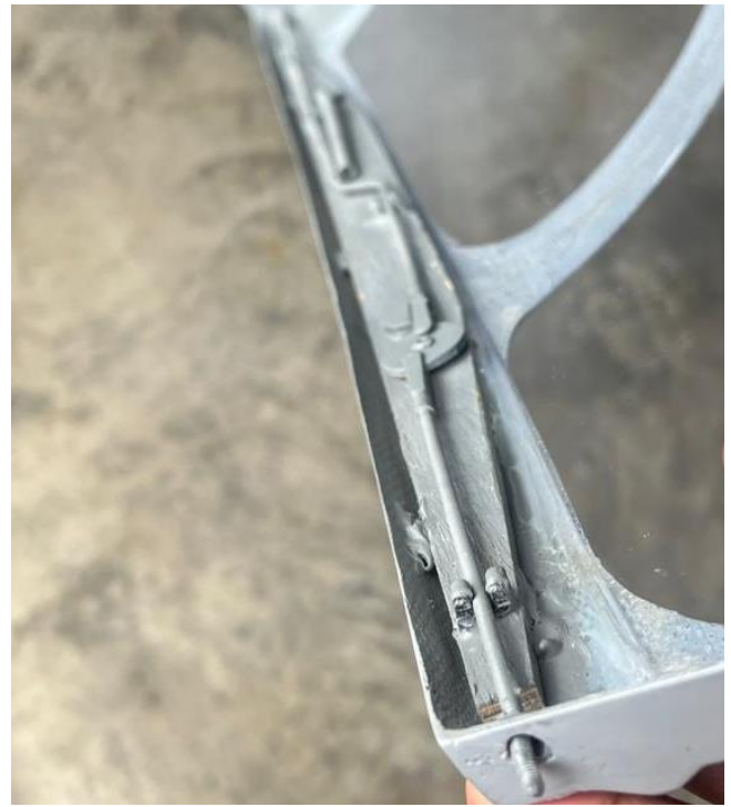
Above: opening and closing system for the canopy set (front part) with front latch.
