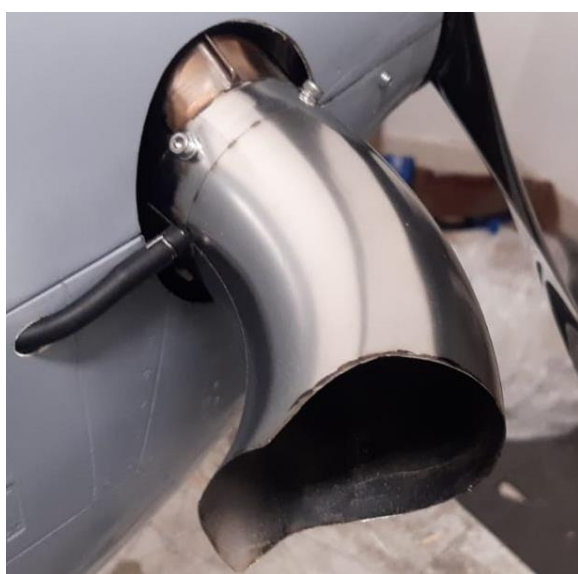
Above: cut exhausts position on turbine for realistic and scale appearance.
