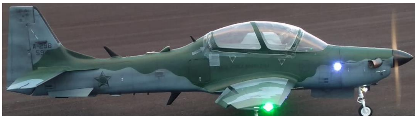
Above: position of the intercept headlight on the front right side of the fuselage.
