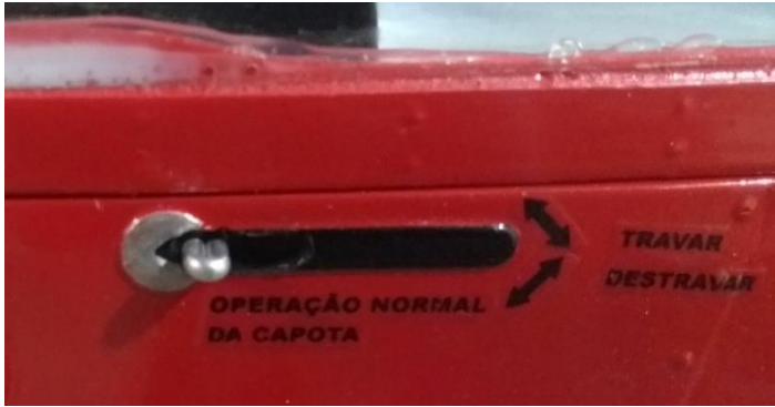
Above: lock position of the canopy / frame assembly on the fuselage.
