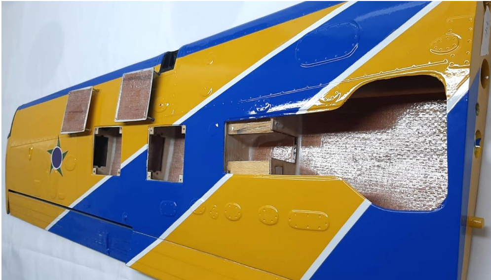
Above: right wing half with open aileron and flap servos compartment covers showing servo fixation points at the ribs.
