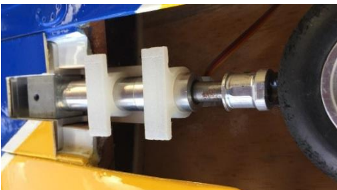
Above: Detail of the fixing of the external door divided into 2 parts with supports on the strut.
