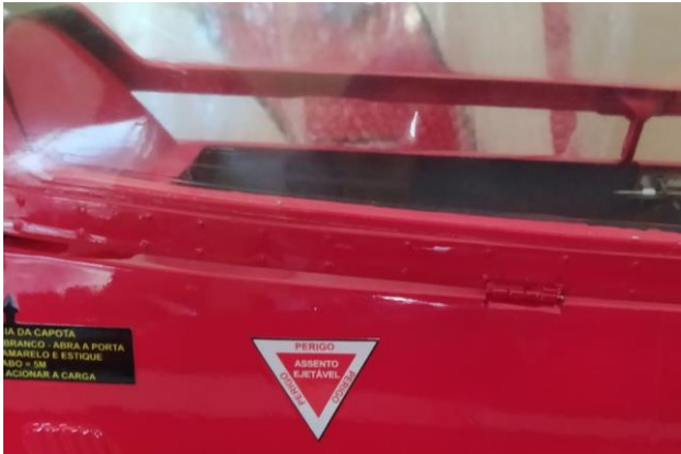
Above: canopy/frame assembly with external Dubro hinges DUB 116.
