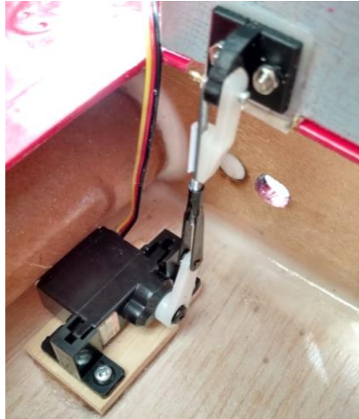
Above: Micro servo installed with linkage and horn for actuation of the mechanism.
