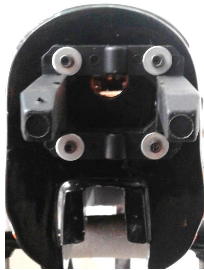
Above: 10-32 blind nuts started to the firewall from the inner side (left) and firewall with screws and washers securing the engine mount (right).
