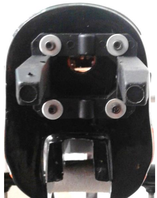
Above: 10-32 blind nuts started to the firewall from the inner side (left) and firewall with screws and washers securing the engine mount (right).
