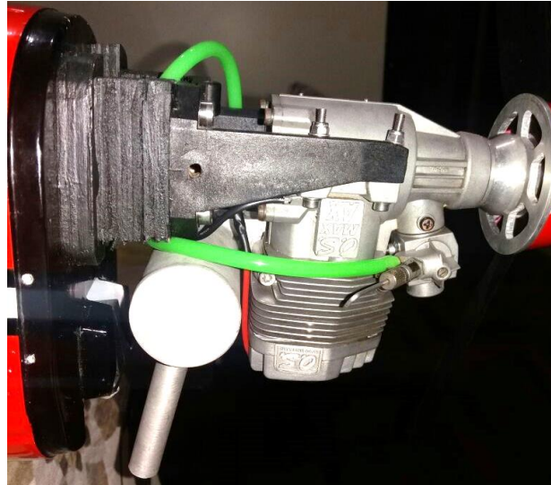
Above: OS 95AX with inverted pitts muffler installation.
