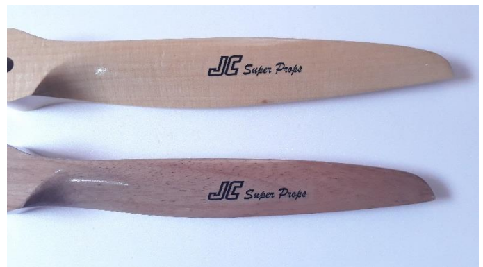
Above: 2 blade wooden propellers for gas burning 20cc engines 14x10 or 15x8.
