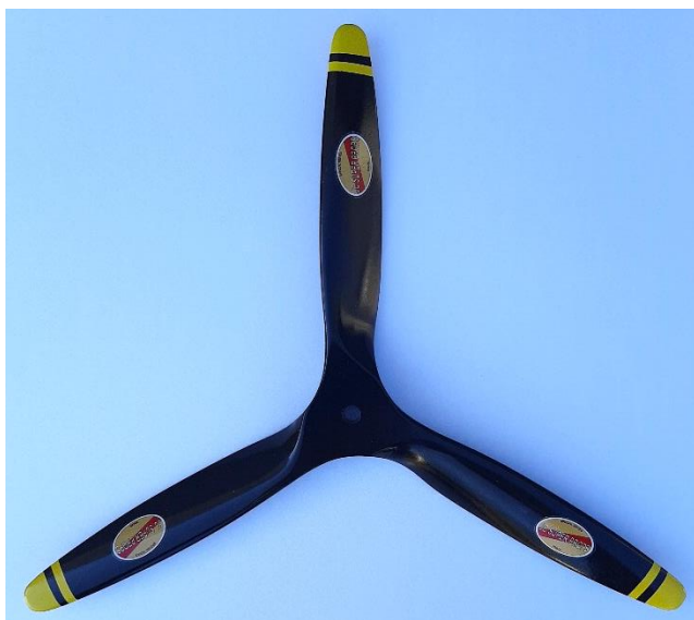
Above: 3 blade 14x9 propellers for gas burning engines (left) and electric motors (right).
