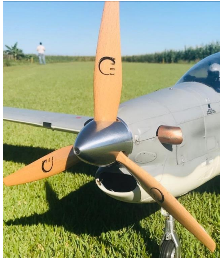
Above: spinner/cowling parallel alignment.
