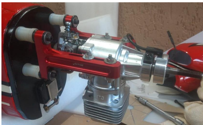
Above: DLE-20RA engine installation on aluminum anti-vibration engine mount.
