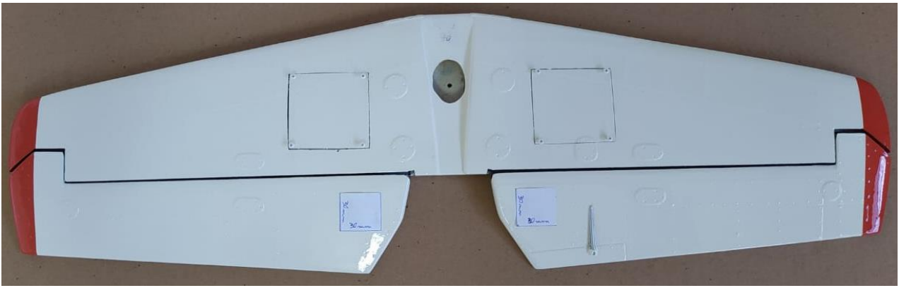
Above: Location of servo access covers and position of elevator horns.
