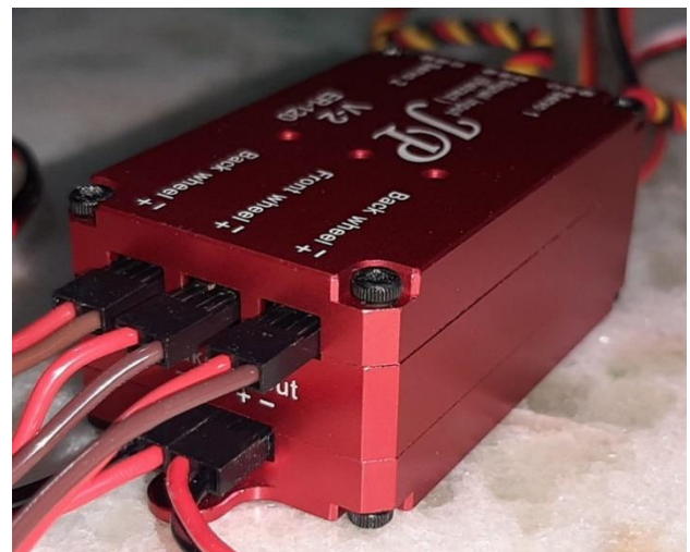
Above: JP ER-120 V2 controller with brakes showing retracts connections on upper side and brakes outputs on lower side. Note the correct polarity of wires as written at controller case.
