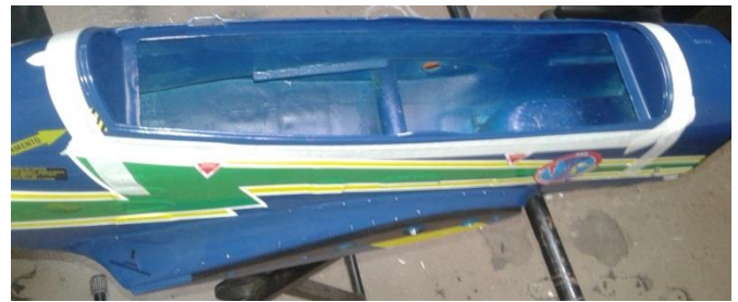
Above: position of the canopy frame on the fuselage and fixing in place with adhesive tape all around.
