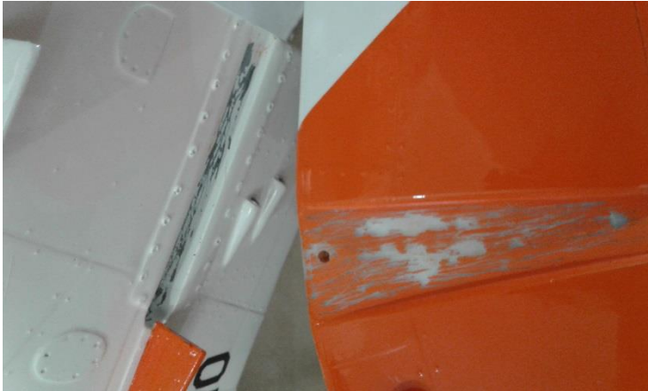
Above: Gluing areas of the stabilizer and fuselage sanded for better adhesion (left) and stabilizer fully inserted into the fuselage (right).
