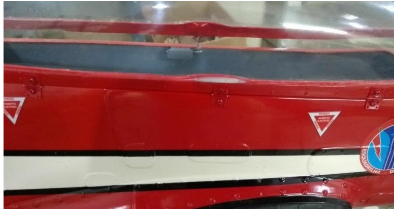
Above: canopy/frame assembly with external Dubro hinges DUB 116.
