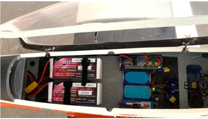
Above: equipment installation examples in the fuselage interior on electric version and Li-Po batteries.
