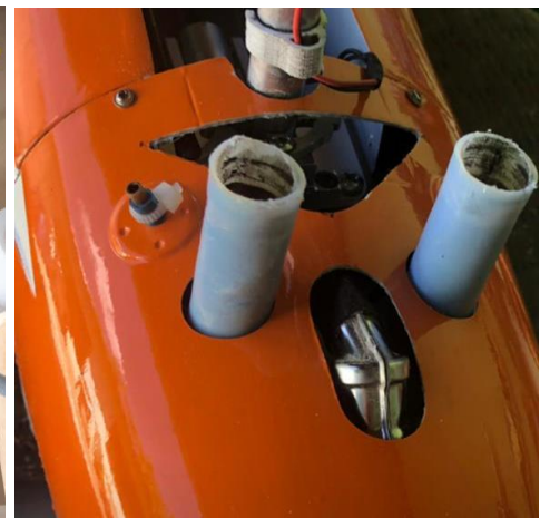
Above: inferior cowling installation with 120 4 cycle glow engine (left and center) and with DLE-20RA muffler exhaust exits and ventilation (right).
