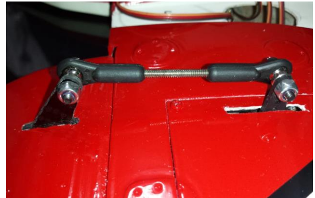
Above: Servo position on stabilizer rib (left) and position of servo arm, horn and elevator command.
