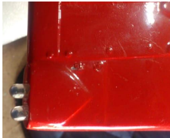
Above: rudder lights board installed at the bottom rear
