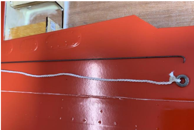
Above: weight on thread tip to pass the wires and wire to pull the wing landing light plates (left).
