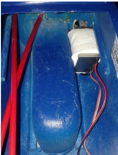
Above: installation of the ignition module behind the firewall on the side and flexible Dubro pushrods for throttle and choke control (left) and engine positioned correctly on the correct alignment (right).
