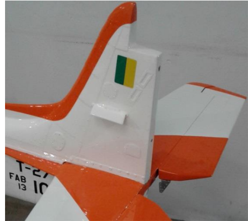
Above: Gluing areas of the stabilizer and fuselage sanded for better adhesion (left) and stabilizer fully inserted into the fuselage (right).
