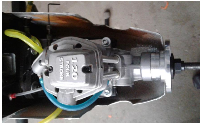
Above: 120 4 cycle engine installation on Great Planes 60-120 adjustable engine mount.
