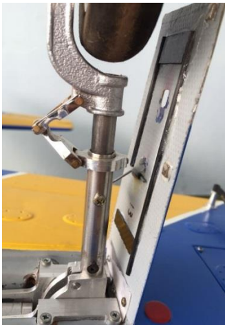
Above: Detail of the attachment of the hinged brackets to the external landing gear door and the closed external landing gear door.
