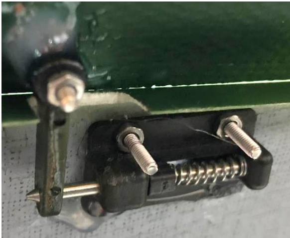
Above: locking the canopy assembly / canopy frame inside the fuselage..
