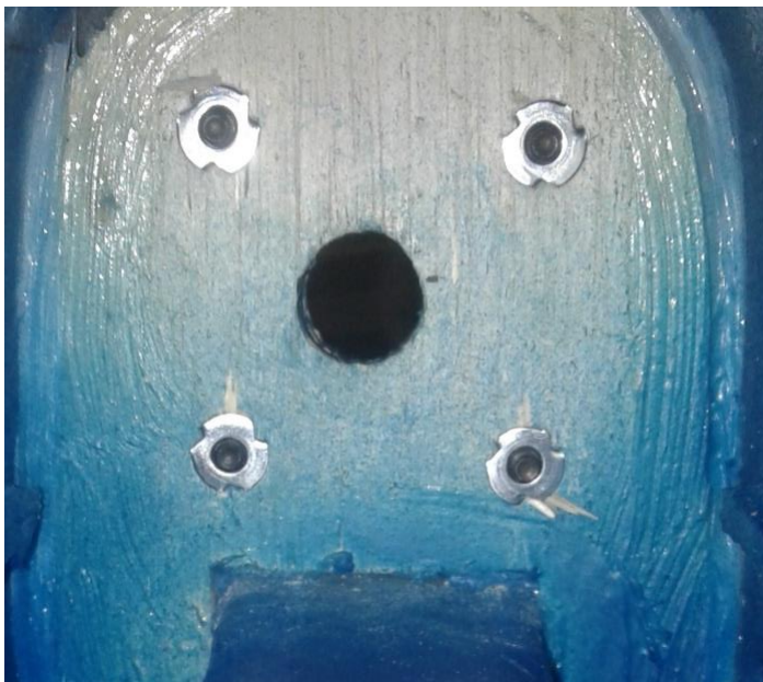
Above: 10-32 blind nuts started to the firewall from the inner side (left) and firewall with screws and washers securing the engine mount (right).
