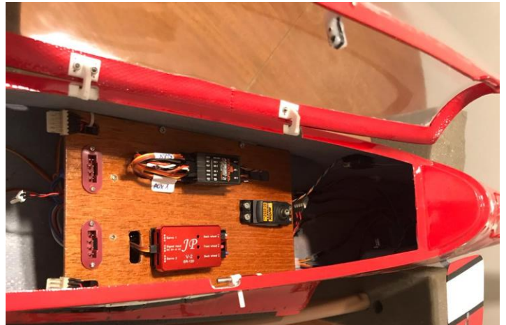
Above: canopy/frame assembly with internal hinges.
