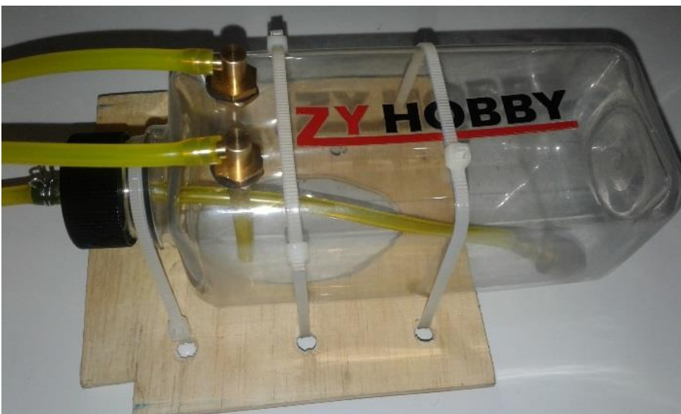
Above: fuel tank with tygon tubes fixed to the fuel tank tray with nylon ties (left) and positioned on rails inside the front of the fuselage (right).
