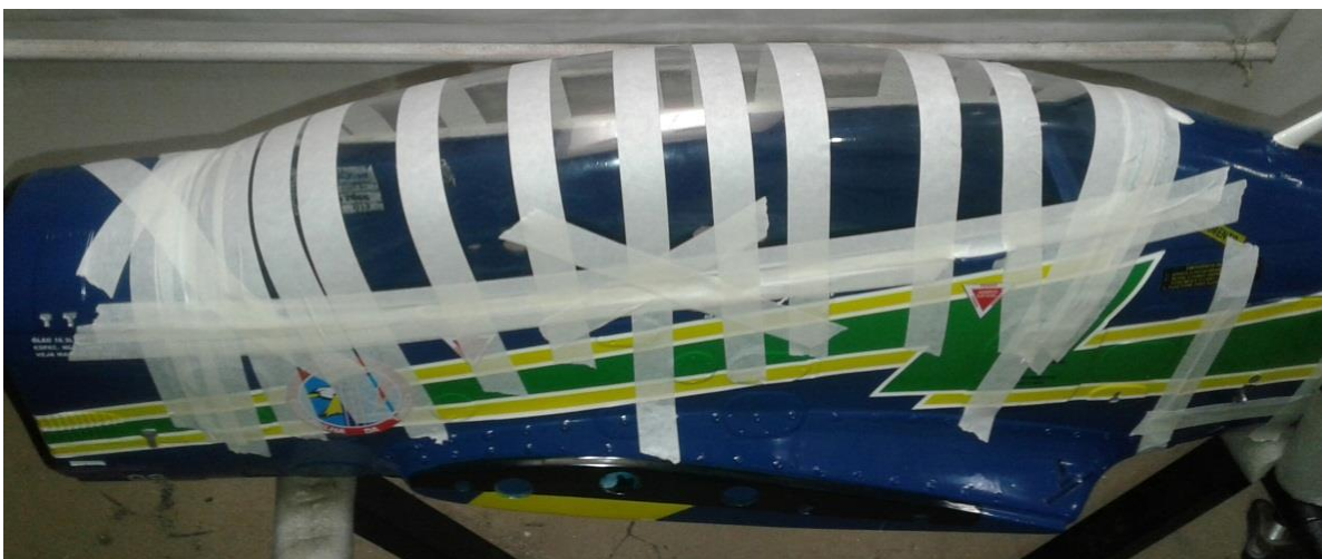
Above: canopy and frame position in the fuselage fixed in place with adhesive tape all around it and also vertically, in order to obtain the correct position between the 3 pieces.
