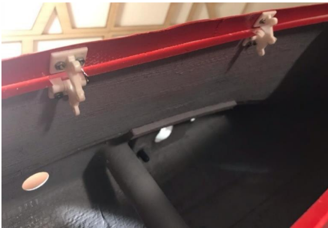
Above: canopy/frame assembly with internal hinges.
