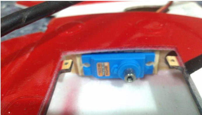
Above: Servo position on stabilizer rib (left) and position of servo arm, horn and elevator command.
