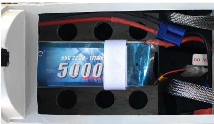
Above: Li-Po batteries used in electric motorization. Final position to be defined after correct C.G. balance.
