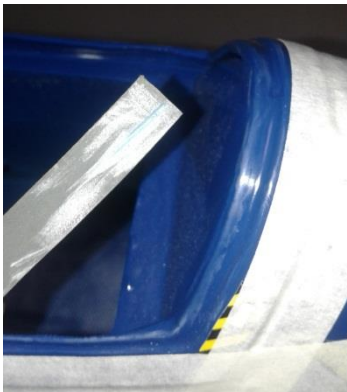
Above: Sand the contact area of the frame to increase glue adhesion (left) and apply white glue to the entire contact area (right).
