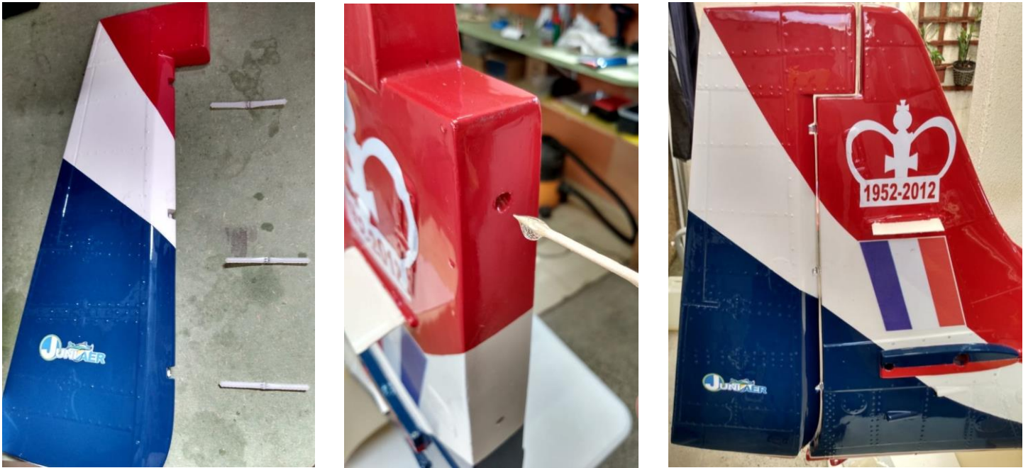
Above: Sequence of gluing the rudder hinges with epoxy glue.
