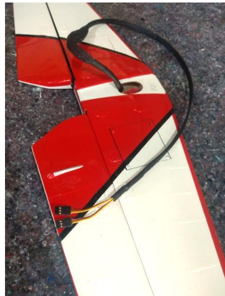
Above: Servo position on the stabilizer rib (left) and elevator servo extensions passing through the lower center of the stabilizer (right).
