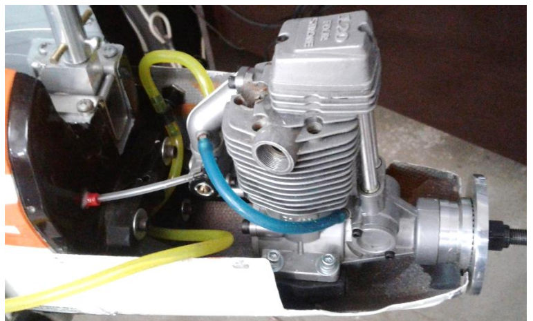
Above: 120 4 cycle engine installation on Great Planes 60-120 adjustable engine mount.
