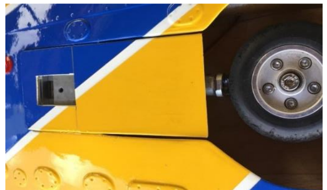
Above: Detail of the fixing of the external door divided into 2 parts with supports on the strut.
