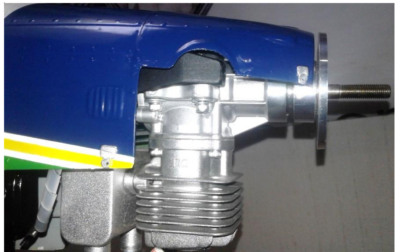
Above: installation of the ignition module behind the firewall on the side and flexible Dubro pushrods for throttle and choke control (left) and engine positioned correctly on the correct alignment (right).
