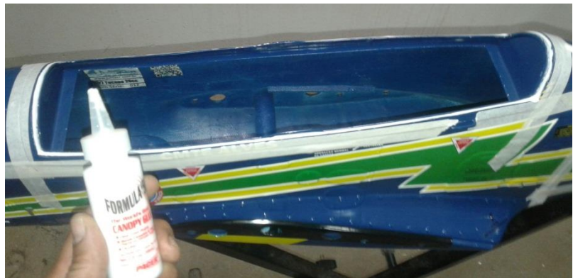
Above: Sand the contact area of the frame to increase glue adhesion (left) and apply white glue to the entire contact area (right).
