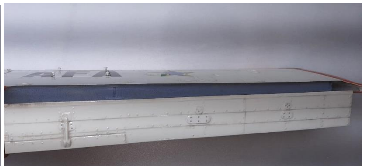
Above: gray areas (trailing edges) on ailerons (right) and flaps (left) shall not be drilled or cut.
