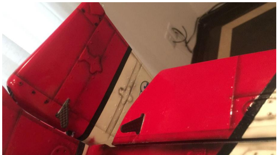
Above: stabilizer and rudder in final position (left) and rudder and elevator control horns (right).
