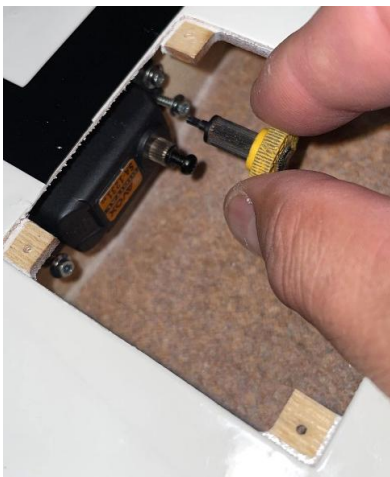
Above: short screwdriver and correct position to screw the wing's servos.
