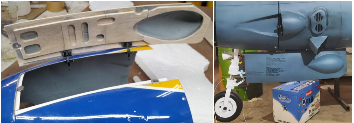
Above: Position of installed front landing gear door and hinges.
