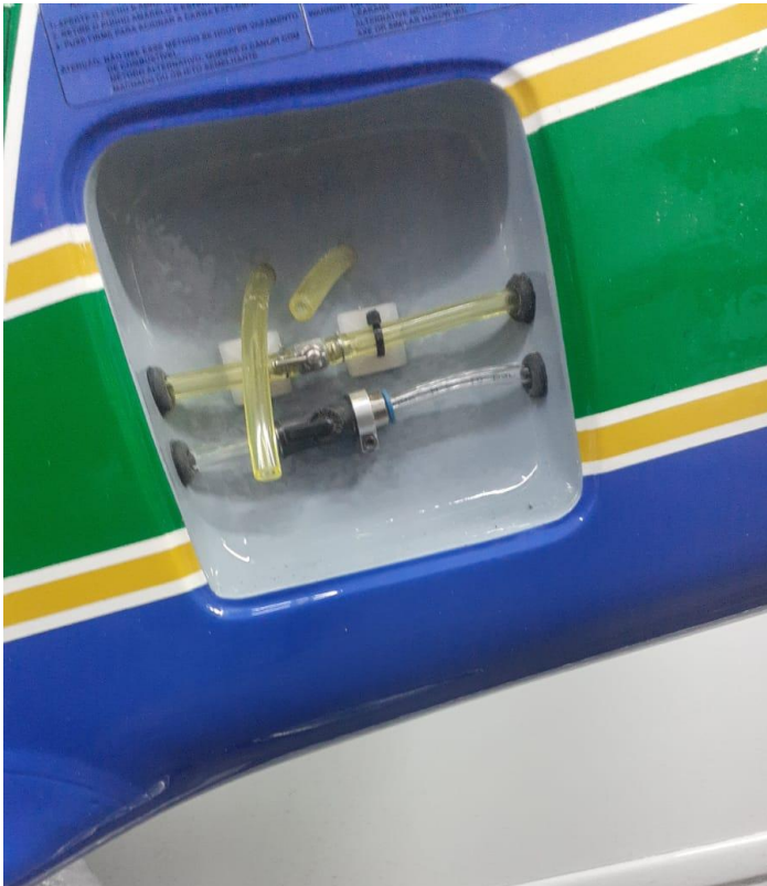
Above: installation of the fuel hoses in the fuselage with connections in the side door of the fuselage (left) and rear tank position on the bottom of the fuselage (right).
