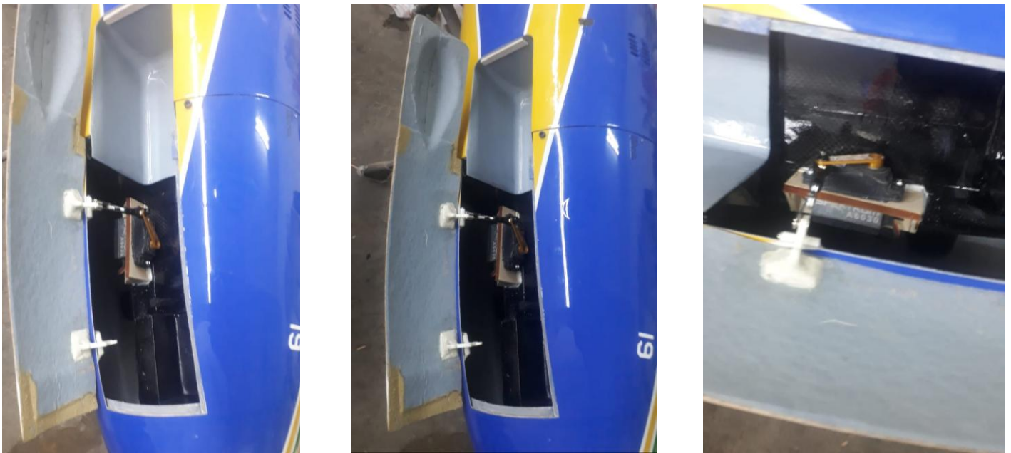
Above: the front landing gear door installed with a Spektrum A6030 servo and 2 hinges.
