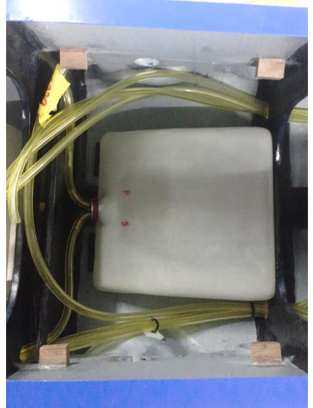
Above: installation of the fuel hoses in the fuselage with connections in the side door of the fuselage (left) and rear tank position on the bottom of the fuselage (right).
