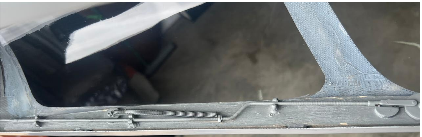
Above: opening and closing system for the canopy set (rear part).
