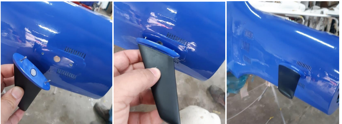
Above: fuselage low antenna installation with magnet and 2-pin.
