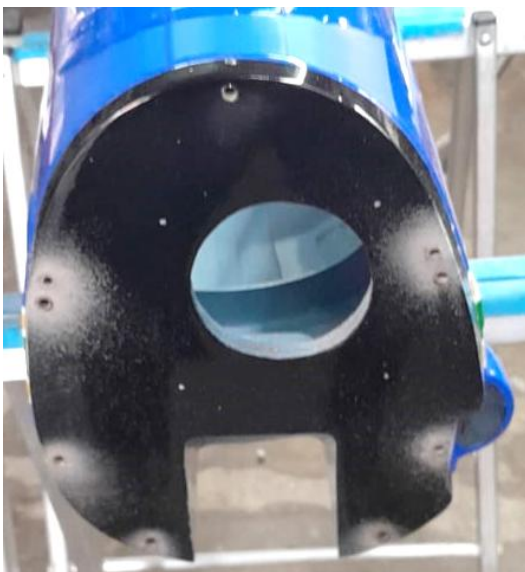
Above: markings of the 4 holes for fixing the turbine mount in the central part of the firewall and 9 holes for fixing the cowling with stud bolts at the ends of the firewall (left and center) and lower fairing attached to the fuselage (right).
