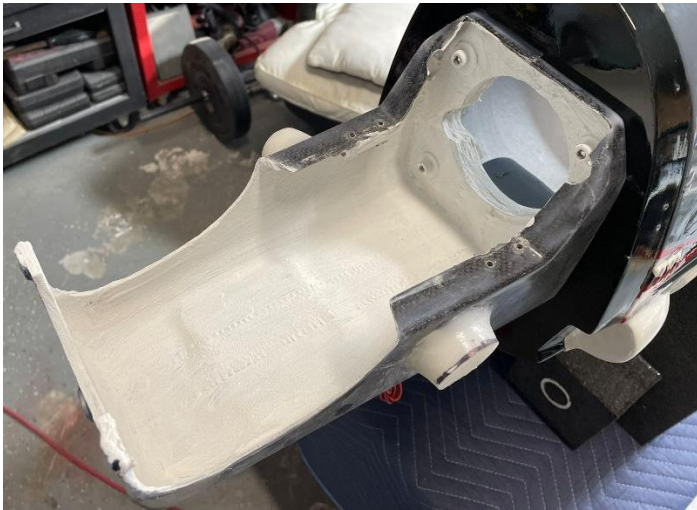
Above: 3 thermal protection paint layers applied on the carbon fiber turbine mount.
