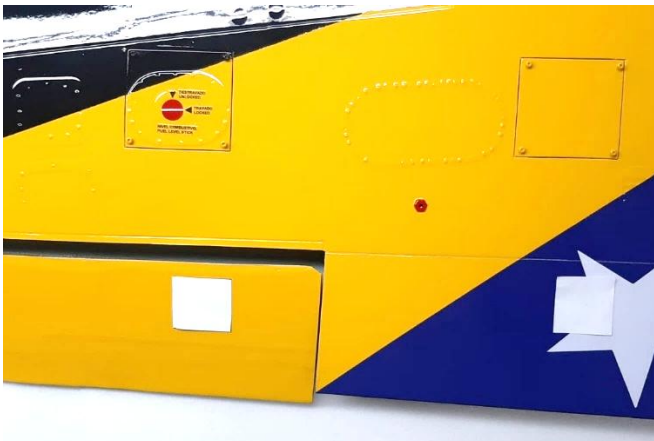
Above: location of the 40mm x 40mm reinforcements for fixing the horns on the right wing (left photo) and positioned and glued horns on the left wing (right photo).
