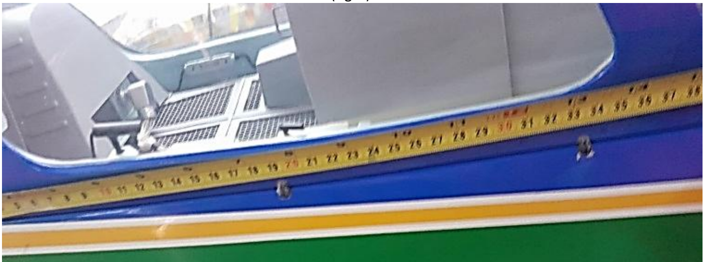
Above: The recommended distance from the rear of the canopy to the rear hinge is 19.5 cm and to the front hinge 33.5 cm.
