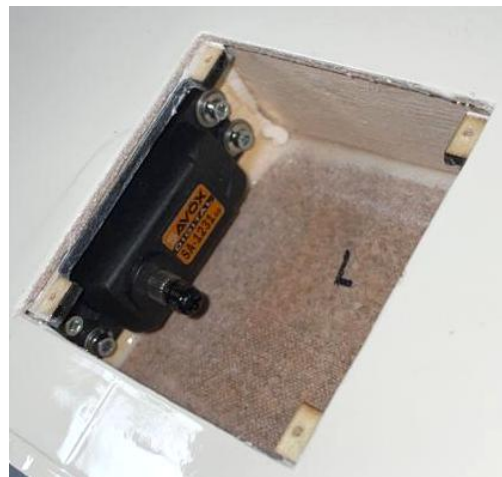
Above: short screwdriver and correct position to screw the wing's servos.
