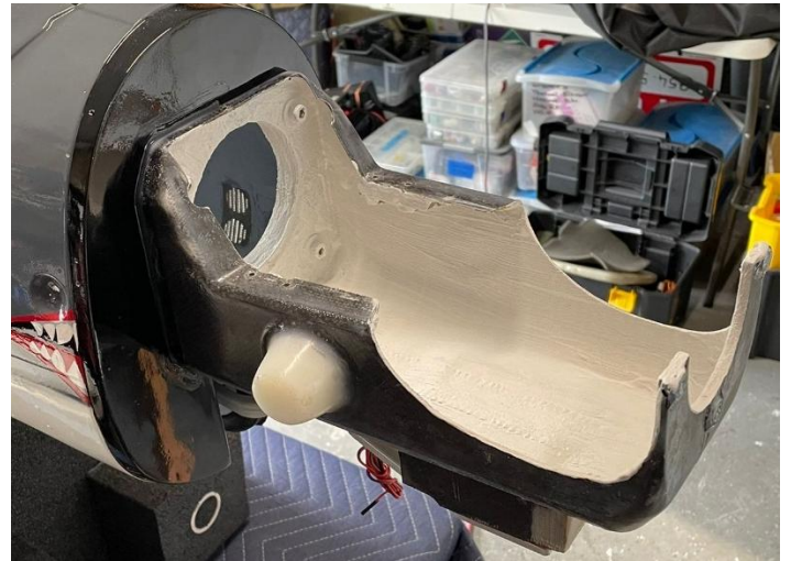
Above: 3 thermal protection paint layers applied on the carbon fiber turbine mount.
