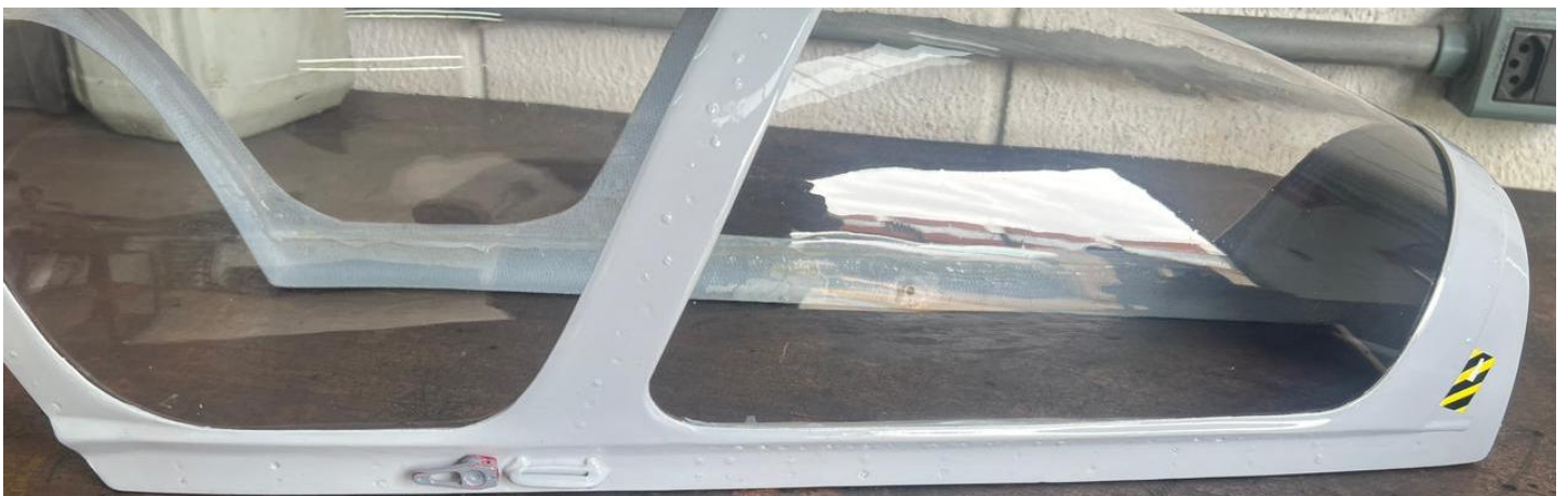
Above: external latch for opening and closing the canopy set.
