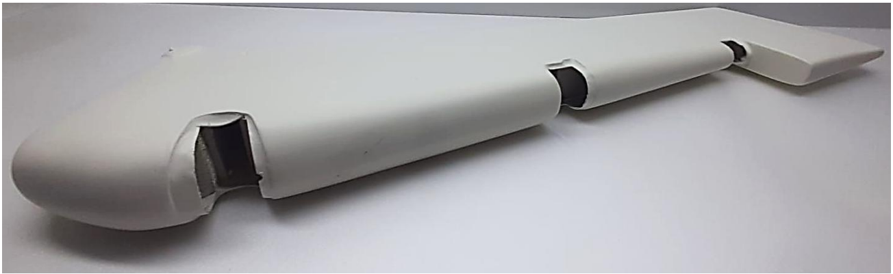
Above: rudder hinges housings.
