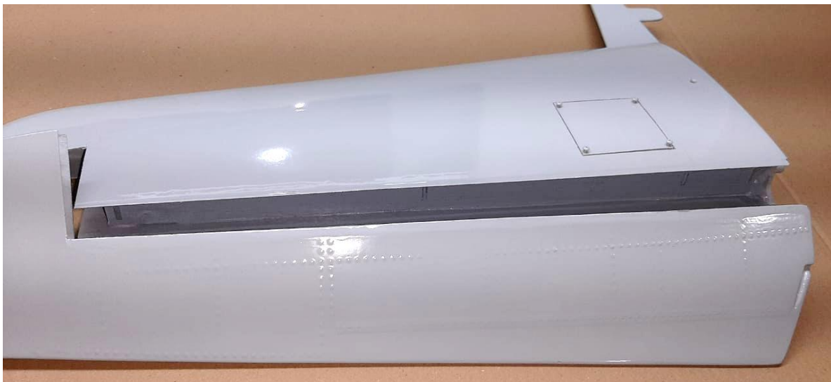
Above: gray areas (trailing edges) on stabilizer shall not be drilled or cut.
