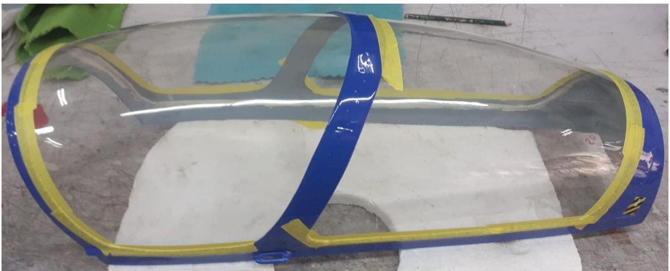
Above: rear part of the clear canopy and canopy frame gluing.
