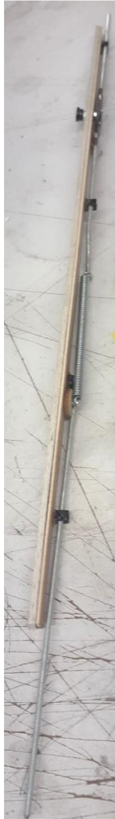
Above: opening and closing system for the canopy set with latches on the front and back in 3 views before installation on cockpit frame.
