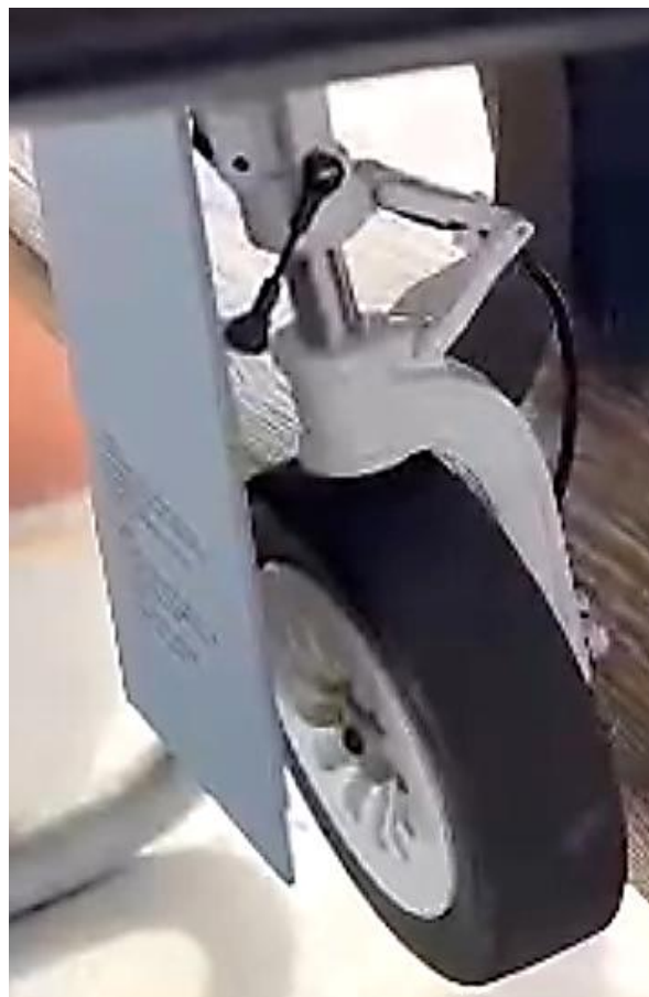
Above: right main landing gear and landing gear door connection made with a pushrod and 2 ball links in the front part of the retract.
