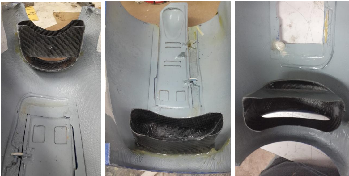
Above: position of gluing the ventilation nozzle to the lower cowling and the cutout at the rear of the nozzle to allow the passage of part of the air flow directly to the rear.
