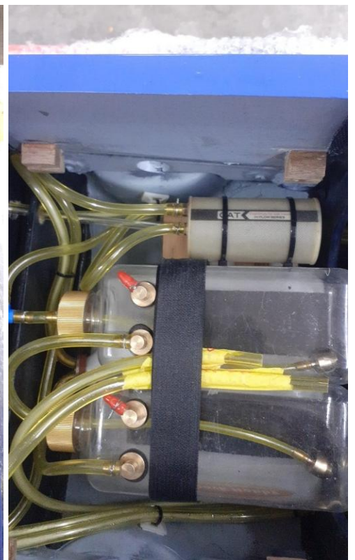
Above: 2 500ml smoke fluid tanks installation above the rear fuel tank (left) and UAT on right also above the rear fuel tank (center and right).
