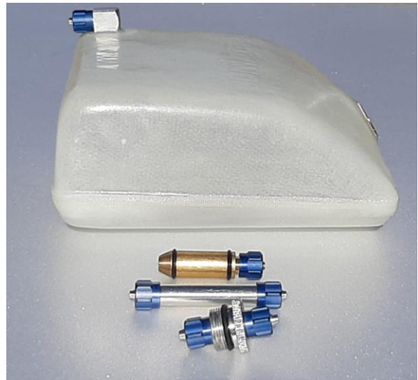
Above: fuel tank with nozzle and air vent installed and internal connections with cover.
