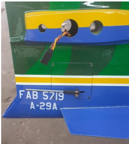
Above: rudder servo position inside the fuselage (left), servo arm linkage (center) and complete linkage with double HD horns(right).
