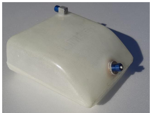
Above: fuel tank with nozzle and air vent installed and clunk assembly with extender and cover (left) and fully assembled fuel tank ready for installation on model airplane (right).
