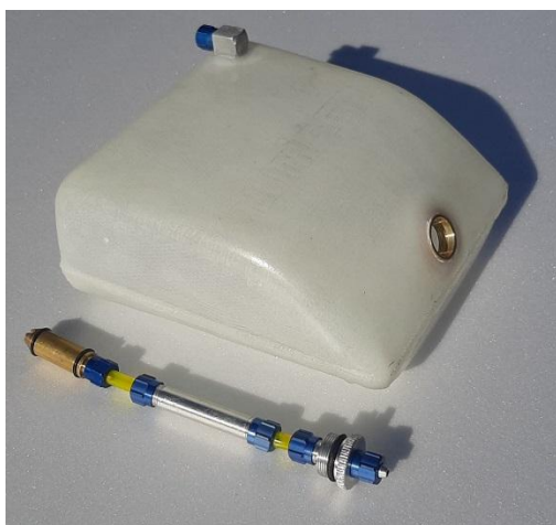
Above: fuel tank with nozzle and air vent installed and clunk assembly with extender and cover (left) and fully assembled fuel tank ready for installation on model airplane (right).
