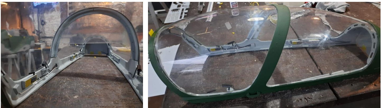
Above: position of the cockpit splitter after installation (left) and rear of the canopy with the 2 sides, central frames and rear trim (right).
