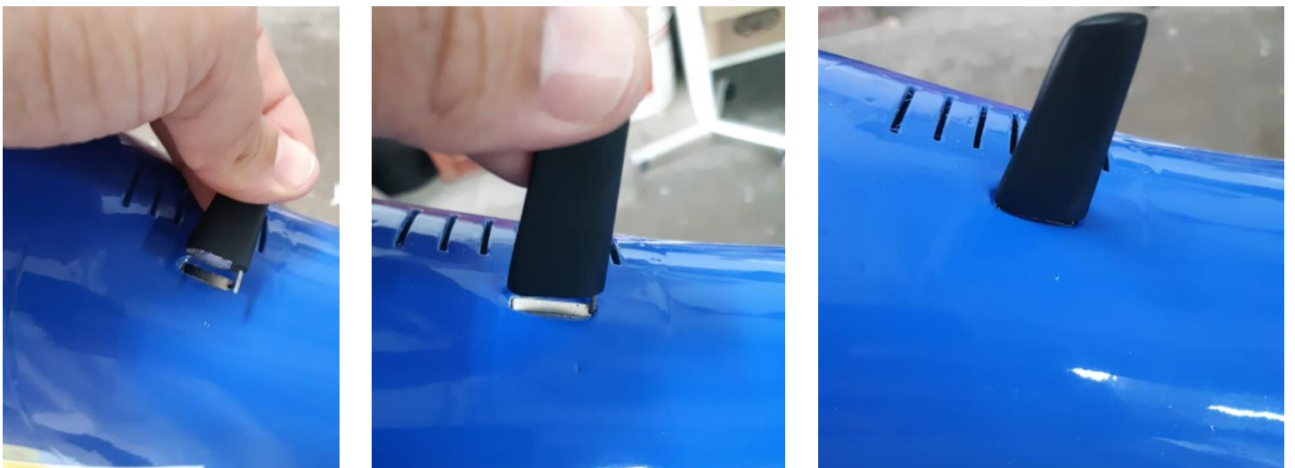
Above: fuselage small top antenna installation with magnet and 2-pin.
