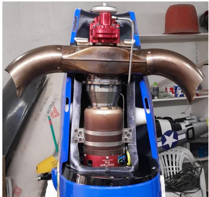
Above: position of the turbine mount on the firewall with lower cowling (left) and the turbine with exhausts fixed to the turbine mount and the firewall with lower cowling (right).
