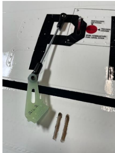
Above: aileron and flaps horns gluing process. Open slots (left), horns position with installed LED linkage (center) and glued horns on aileron command surface (right).
