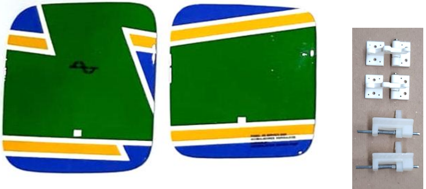
Above: right side door (bigger, on left), left side door (smaller, on center) and hinges and latches supplied with the kit for side doors installation (right).
