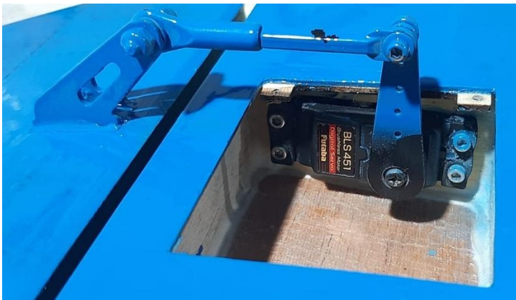
Above: elevators servos, servo arms and horns position with linkage.
