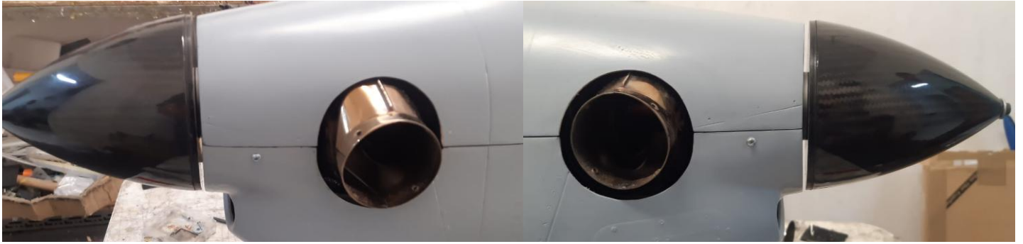
Above: correct alignment of the nose cowling with the spinner assembly and turbine exhausts holes.
