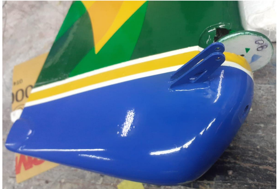
Above: rudder horns position with one-side operation command.
