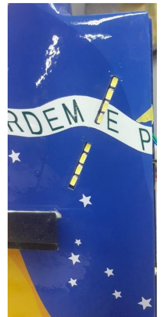
Above: right side of the original vertical stabilizer without cuts (left), cuts on the left side of the vertical stabilizer to allow the installation of formation lights (center) and LEDs properly installed (right).
