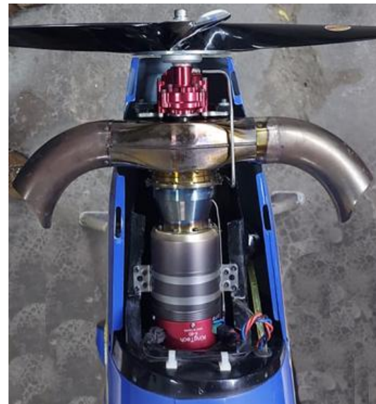
Above: cut exhausts position on turbine for realistic and scale appearance.
