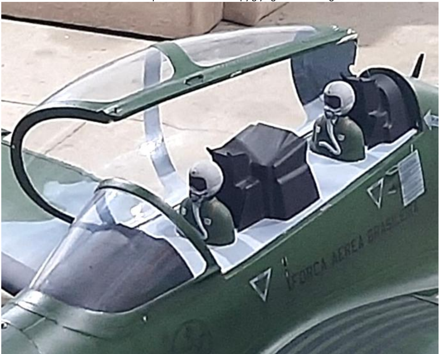
Above: front clear canopy glued to the fuselage and rear canopy glued to the canopy frame with side opening.
