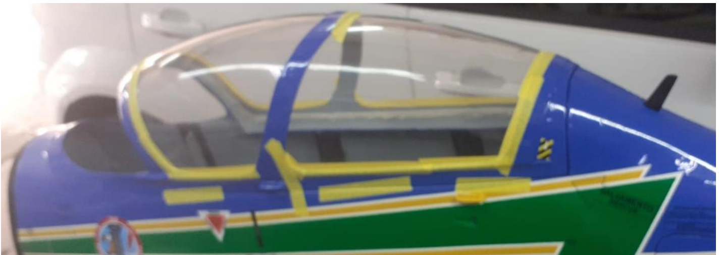
Above: rear part of the clear canopy and canopy frame gluing and curing fixed to the fuselage to get the correct shape.
