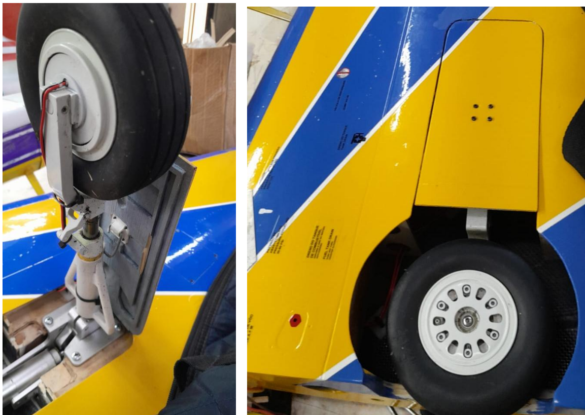
Above: external main landing gear door and hinges position on wing with landing gear door linkage.
