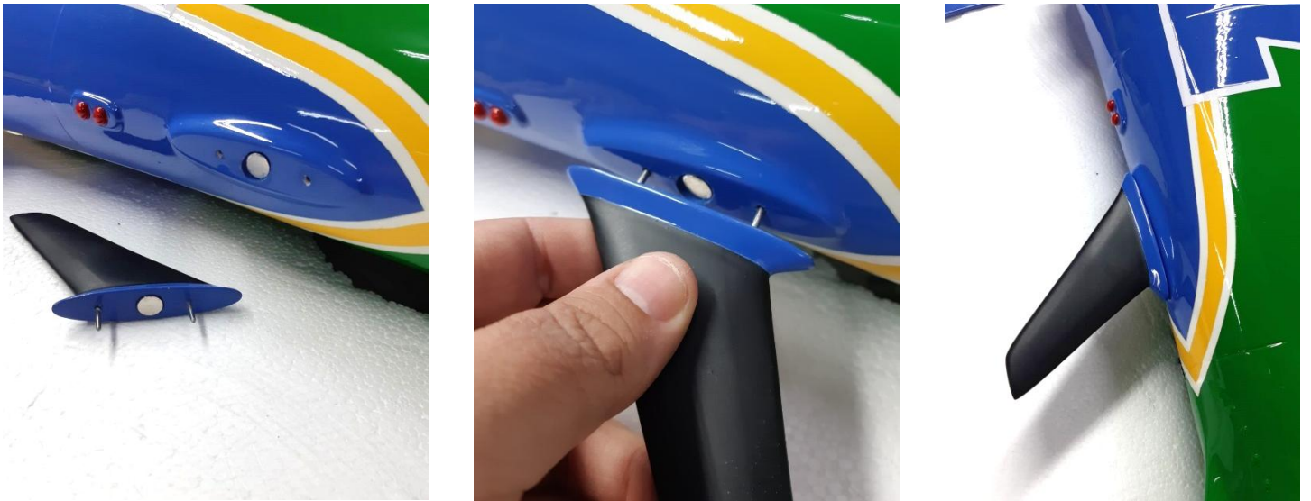
Above: fuselage top antenna installation with magnet and 2-pin.
