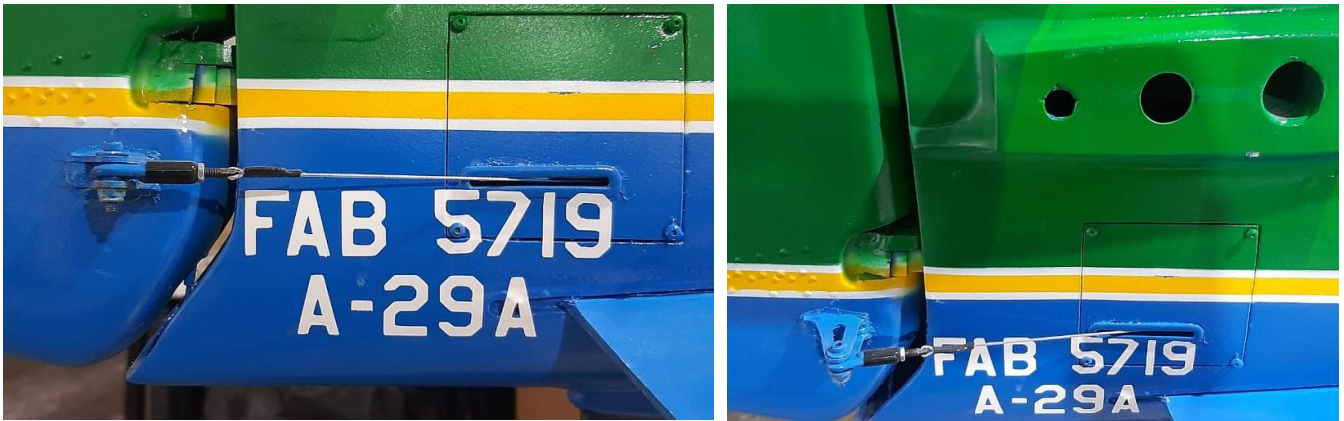
Above: pull-pull steel cables exits, with Dubro heavy duty 4-40 ball links fixed on control horns with 4-40 screws and parlock nuts on both sides of the fuselage.
