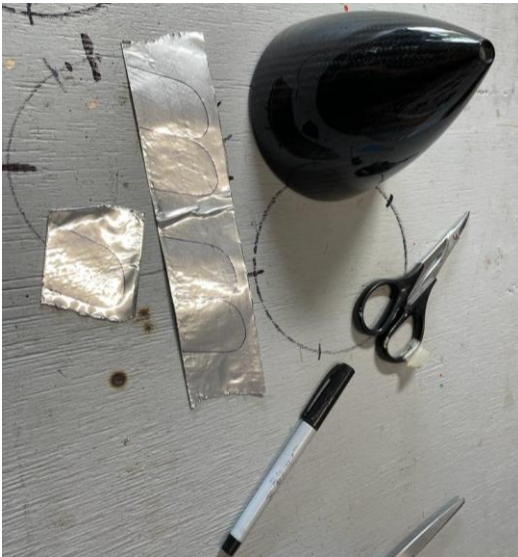
Above: spinner cut sequence to install the 5-blade propeller using equal shape adhesives.
