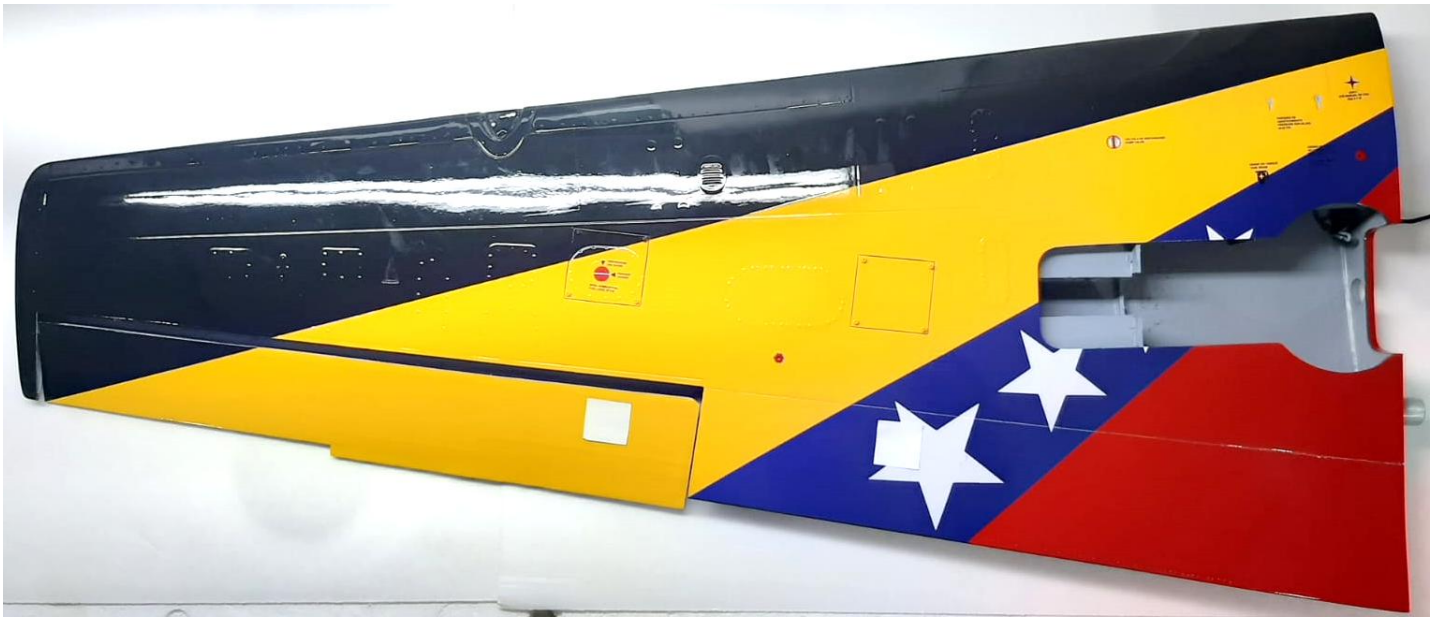
Above: location of the 40mm x 40mm reinforcements for fixing the horns on the right wing.
