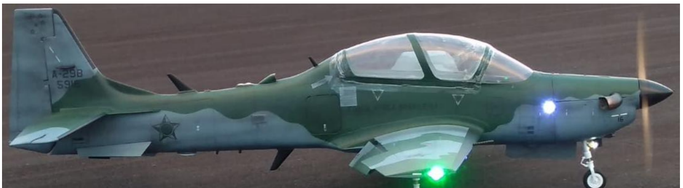
Above: position of the intercept headlight on the front right side of the fuselage.
