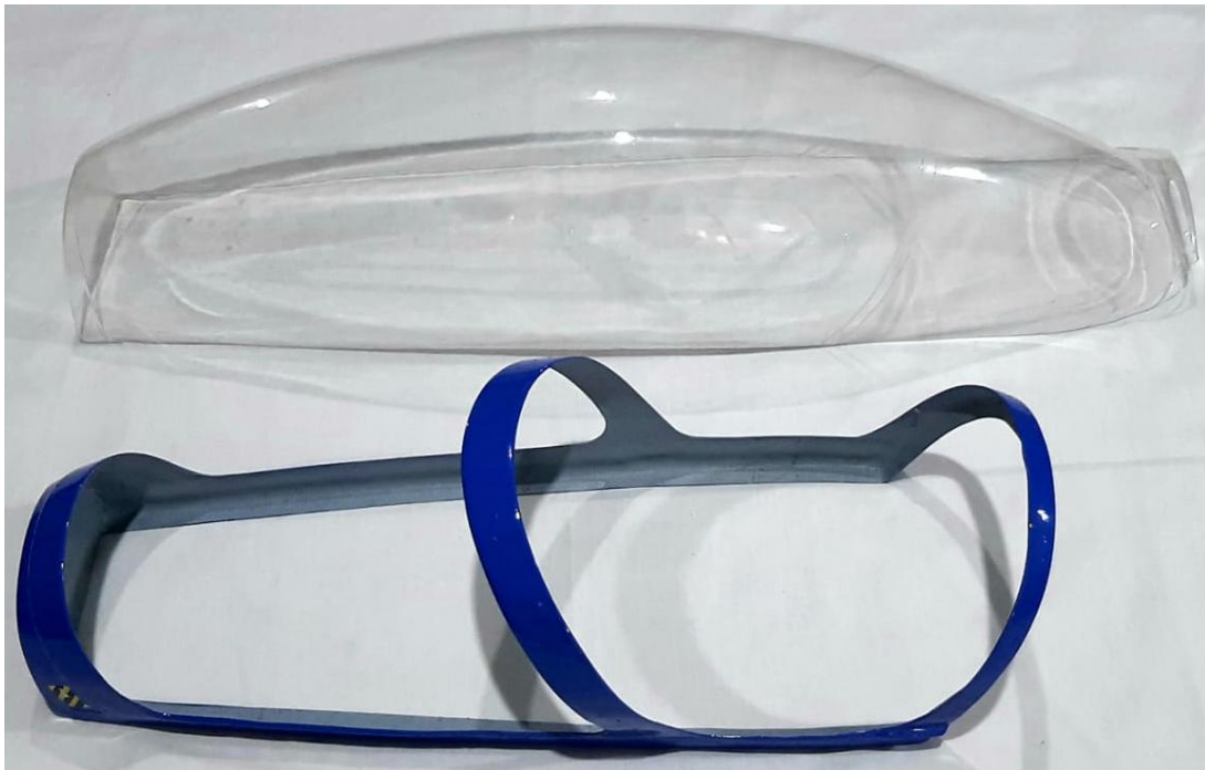
Above: canopy frame that shall be glued from above to the rear part of the canopy.
