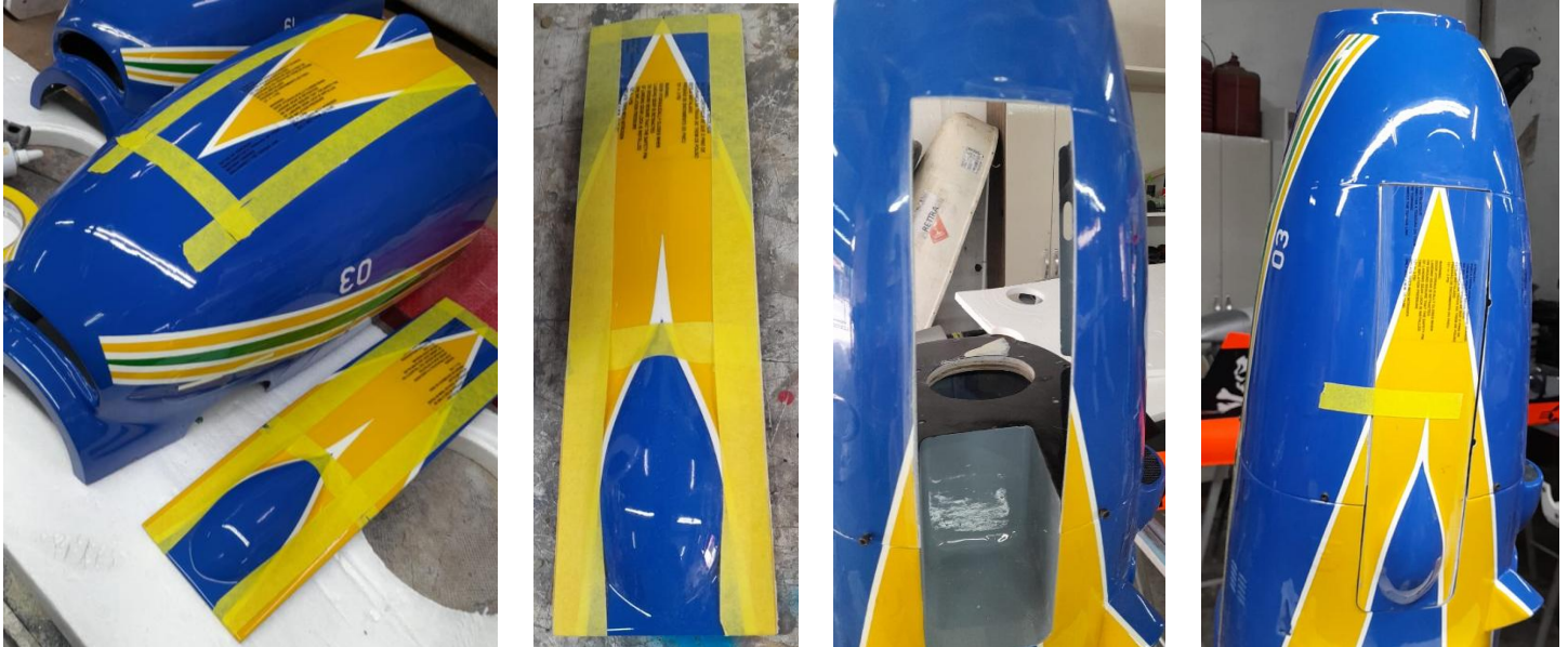
Above: Sequence of cutout of the lower cowling and adjustment of the front landing gear door.
