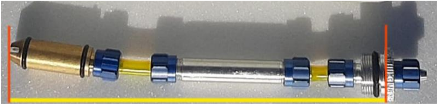
Above: total length of clunk assembly 16,5cm .
