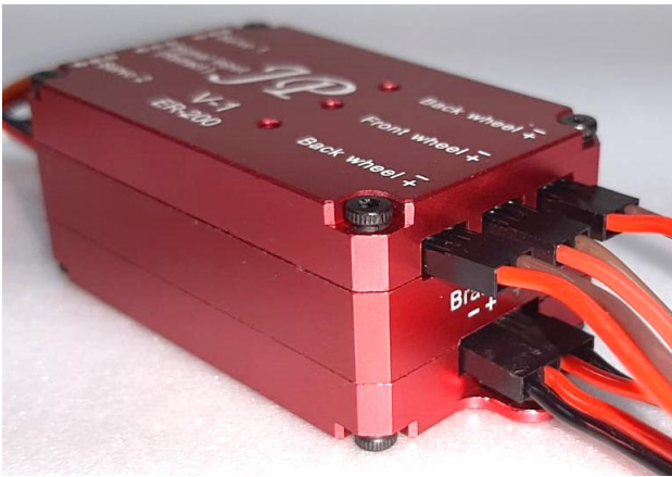
Above: JP ER-200 V1 controller with brakes showing retracts connections on upper side and brakes outputs on lower side. Note the correct polarity of wires as written at controller case.
