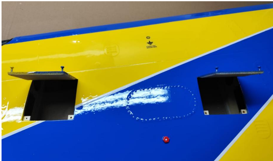
Above: servo compartment access covers location for ailerons and flaps servos and fixation holes on ribs.
