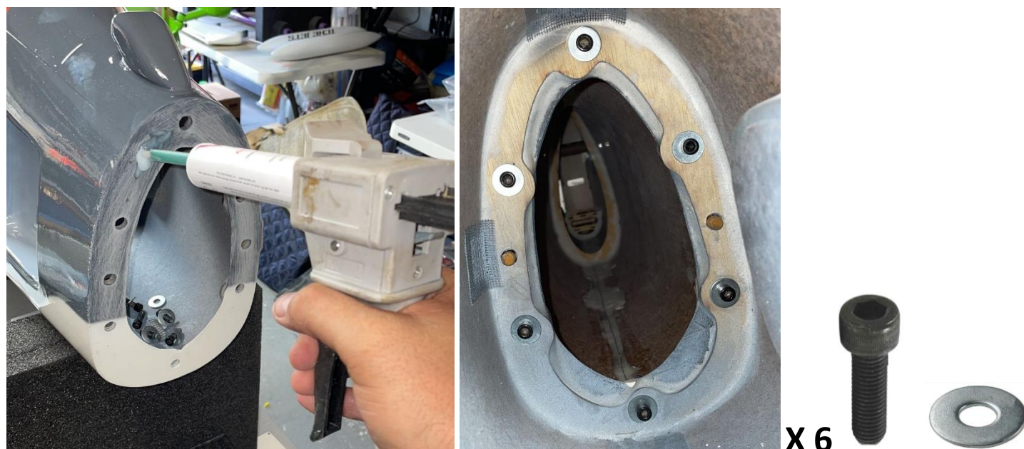
Above: application of epoxy glue on the front section of the fuselage (left), parts joined with screws and washers in the final location (center) and 1/4" x 3/4" allen screw with 1/4" washer to be used ( right).
