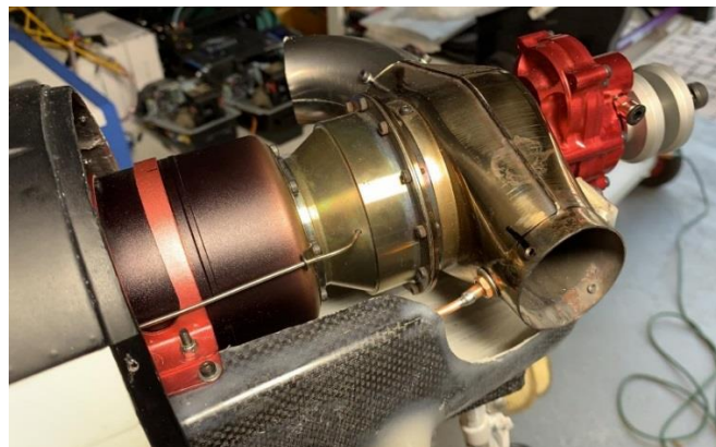
Above: fittings installed showing the flattening at the end of the tube for better spraying of the fluid (left) and final position with complete installation (right).
