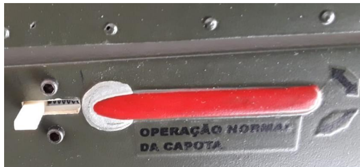
Above: lock position of the canopy / frame assembly on the fuselage.
