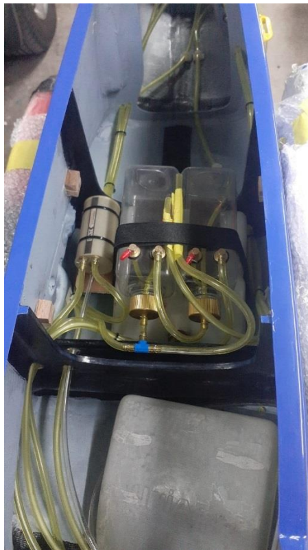
Above: 2 500ml smoke fluid tanks installation above the rear fuel tank (left) and UAT on right also above the rear fuel tank (center and right).
