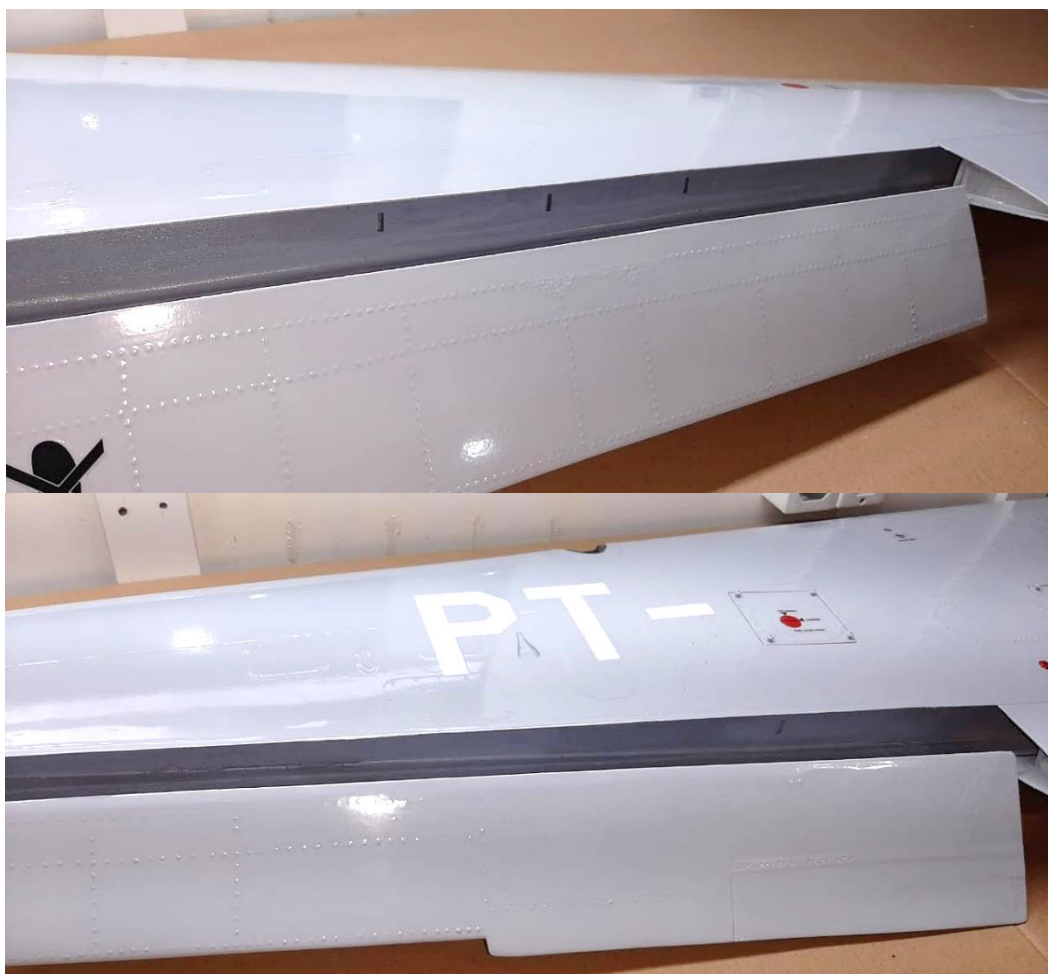
Above: gray areas (trailing edges) on ailerons and flaps shall not be drilled or cut.
