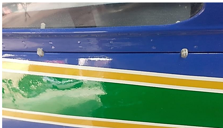
Above: canopy assembly hinges on fuselage (left) and in position for gluing to fuselage and canopy frame (right).
