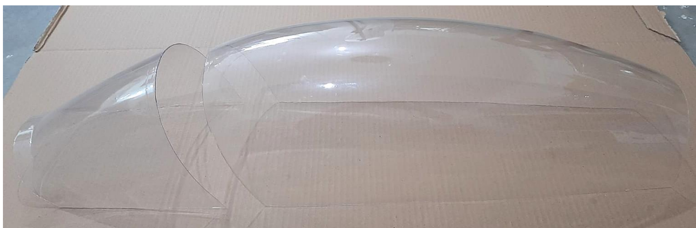
Above: correct desired shape of the 2 canopy parts after cut.
