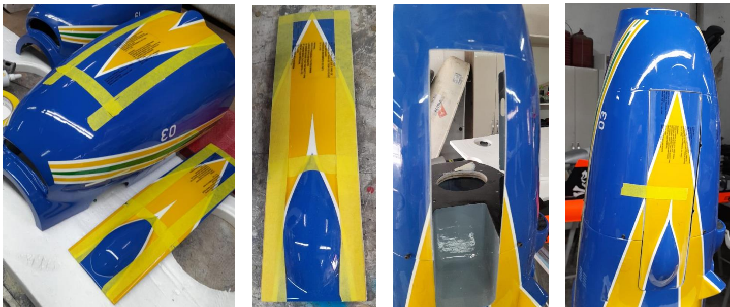
Above: Sequence of cutout of the lower cowling and adjustment of the front landing gear door.
