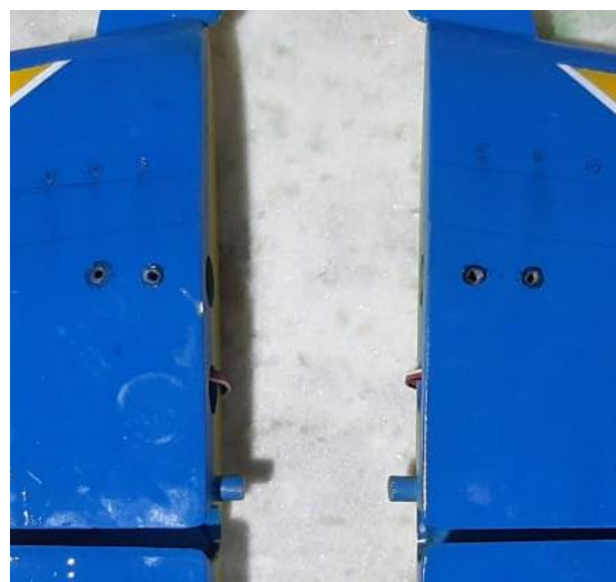
Above: position of the tube in the middle of the stabilizer and fuselage (left) and detail of the holes location for fixing the stabilizer halves in the stabilizer tube (right).
