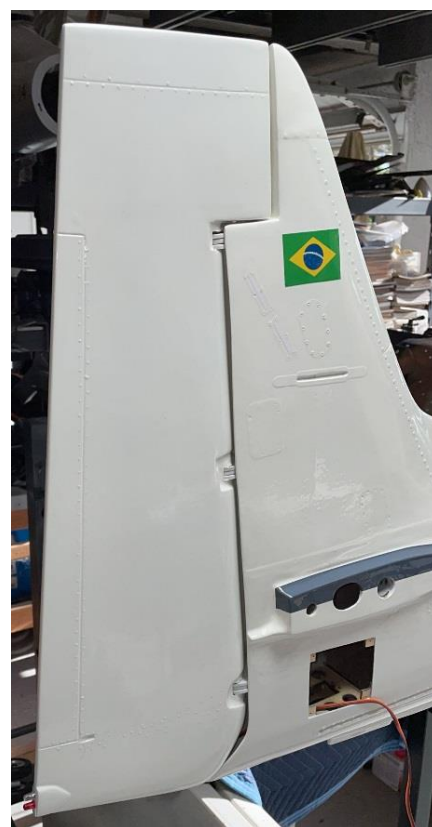
Above: rudder with glued hinges (left), housing for hinges on the vertical stabilizer (center) and rudder glued and installed (right).
