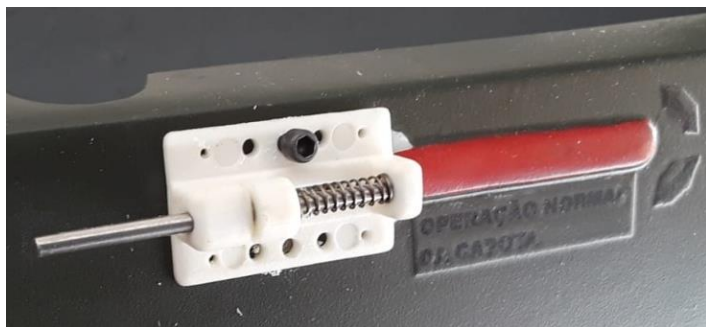
Above: lock position of the canopy / frame assembly on the fuselage.
