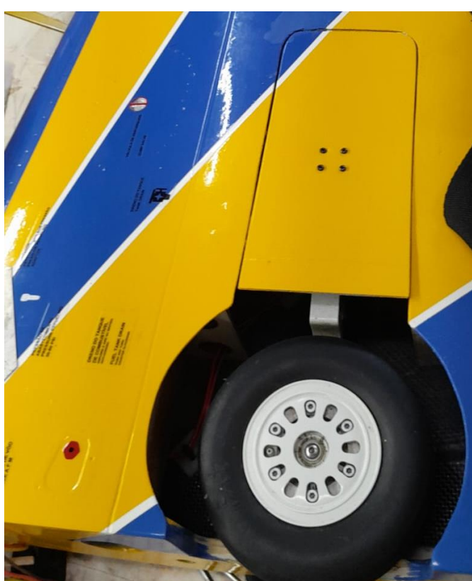
Above: external main landing gear door and hinges position on wing with landing gear door linkage.
