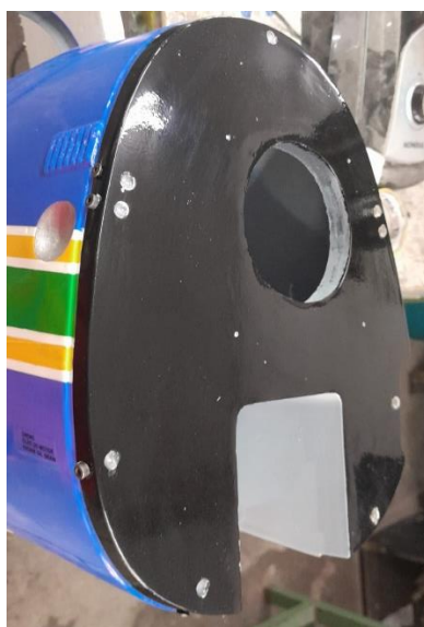
Above: markings of the 4 holes for fixing the turbine mount in the central part of the firewall and 9 holes for fixing the cowling with stud bolts at the ends of the firewall (left and center) and lower fairing attached to the fuselage (right).
