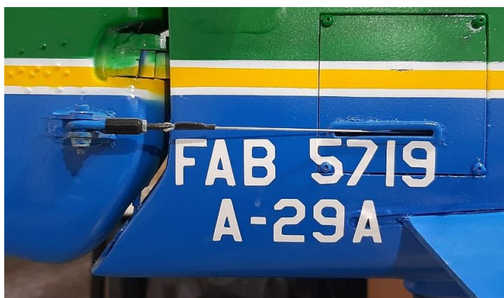
Above: pull-pull steel cables exits, with Dubro heavy duty 4-40 ball links fixed on control horns with 4-40 screws and parlock nuts on both sides of the fuselage.
