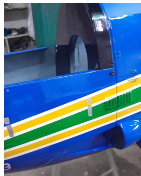
Above: markings of the 4 holes for fixing the turbine mount in the central part of the firewall and 9 holes for fixing the cowling with stud bolts at the ends of the firewall (left and center) and lower fairing attached to the fuselage (right).
