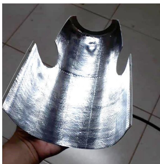
Above: inner part of the upper cowling painted with thermal protection paint and application of a ceramic fiber fabric (left) and a layer of aluminum foil on the outside (right).
