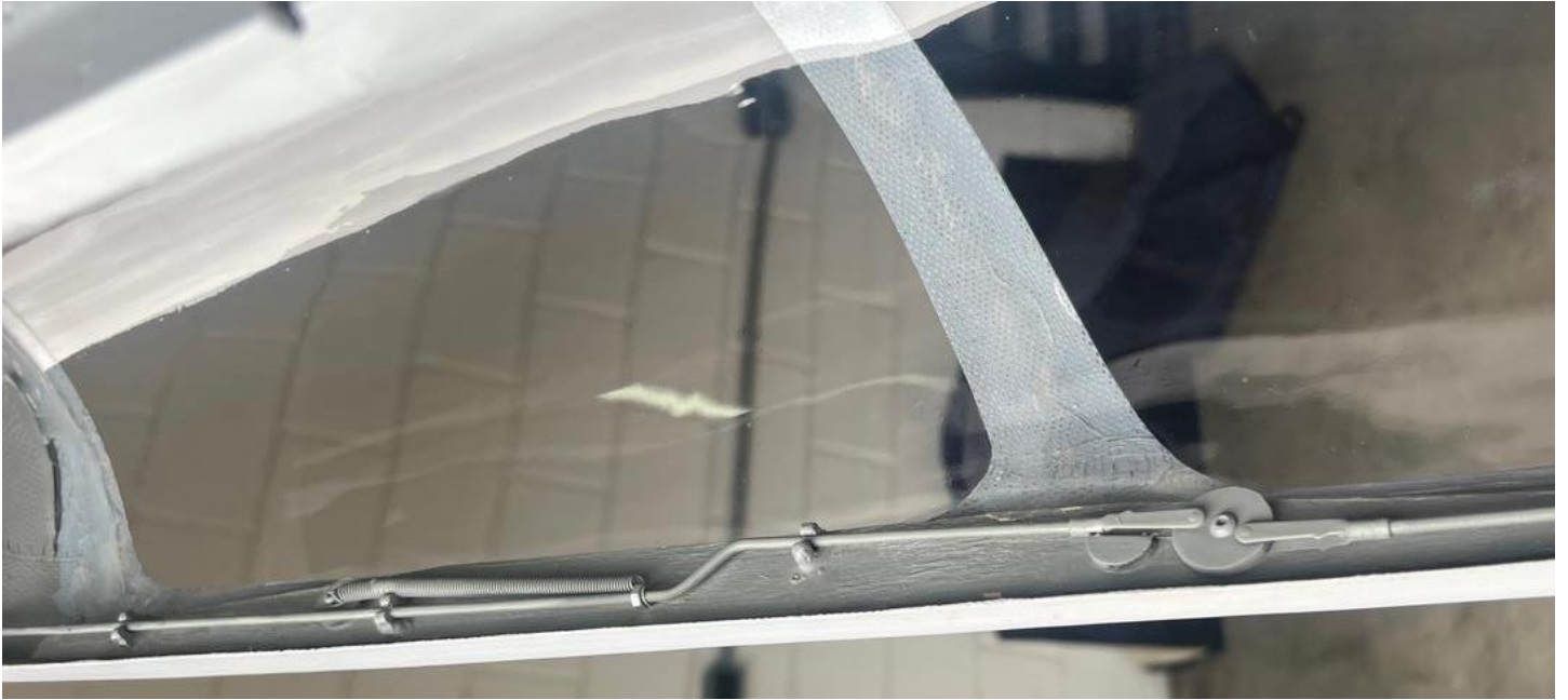
Above: opening and closing system for the canopy set (rear part).
