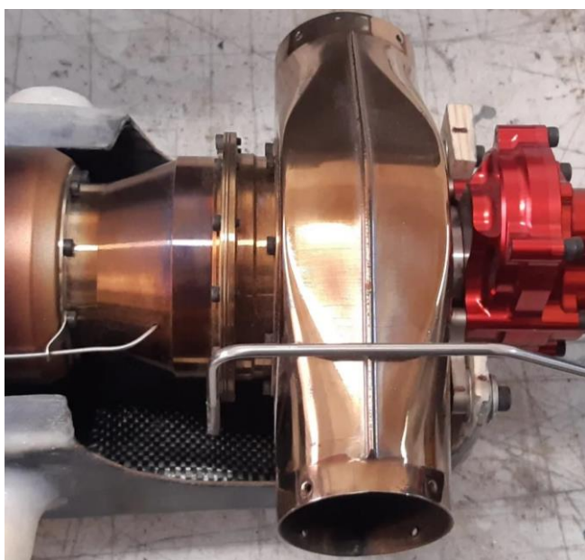
Above: turbine position on the carbon fiber turbine mount and lubrication tube position.
