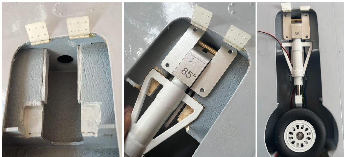
Above: lowering of the main retractable block (wing) to accommodate the triangular shape of the strut.
