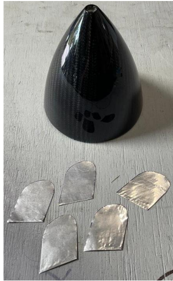
Above: spinner cut sequence to install the 5-blade propeller using equal shape adhesives.
