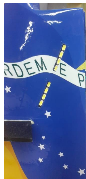
Above: right side of the original vertical stabilizer without cuts (left), cuts on the left side of the vertical stabilizer to allow the installation of formation lights (center) and LEDs properly installed (right).
