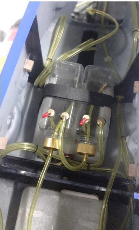
Above: 2 500ml smoke fluid tanks installation above the rear fuel tank (left) and UAT on right also above the rear fuel tank (center and right).
