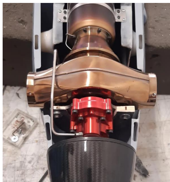
Above: turbine position on the carbon fiber turbine mount and lubrication tube position.
