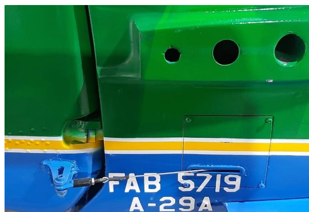
Above: pull-pull steel cables exits, with Dubro heavy duty 4-40 ball links fixed on control horns with 4-40 screws and parlock nuts on both sides of the fuselage.
