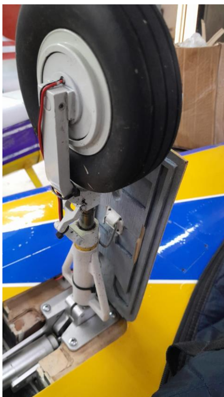
Above: external main landing gear door and hinges position on wing with landing gear door linkage.
