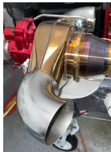
Above: exhausts position installed on turbine.
