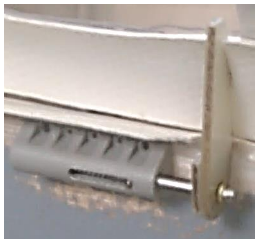
Above: locking the canopy assembly / canopy frame inside the fuselage.
