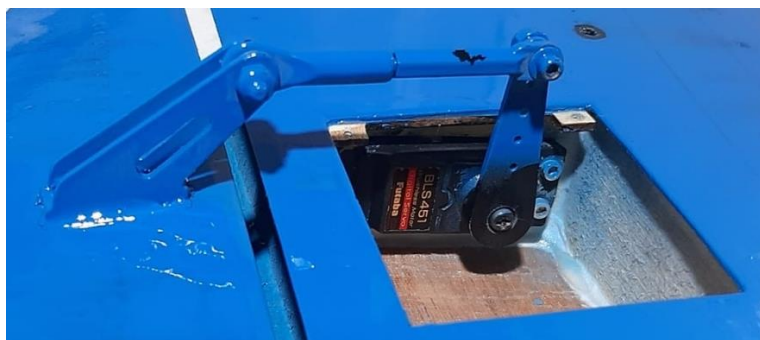
Above: elevators servos, servo arms and horns position with linkage.
