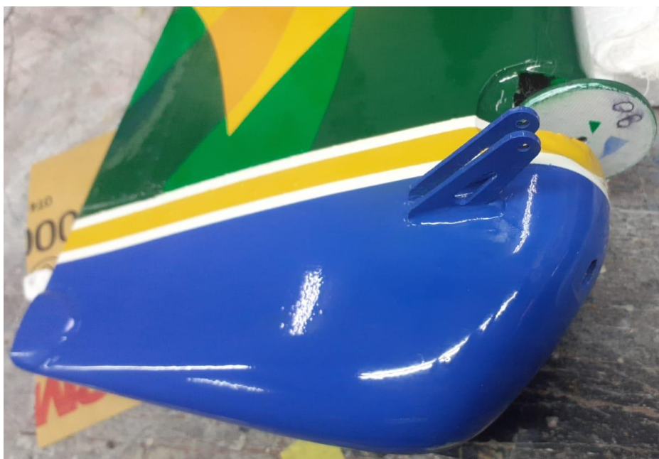
Above: rudder horns position with one-side operation command.
