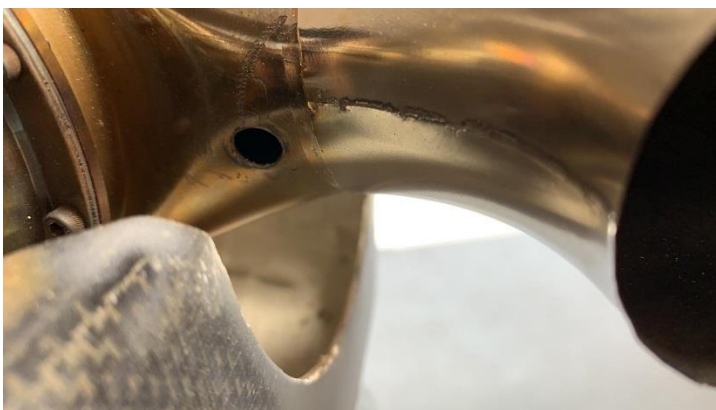
Above: Dubro DUBR 192 connections (left) and hole for installing the connections for smoke fluid in the turbine exhaust body (right).
