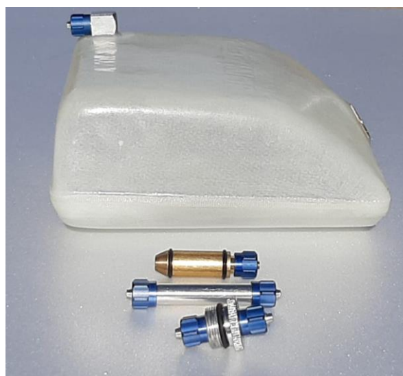
Above: fuel tank with Rio Jets nozzle and air vent installed and internal connections with cover.
